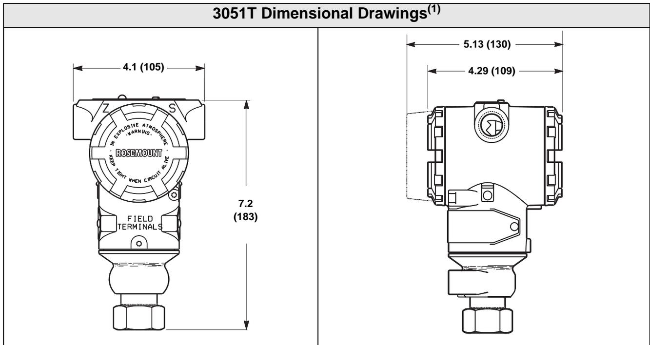
(1) For FOUNDATION fieldbus and Profibus PA transmitters with LCD Display, housing length is 5.36 in. (136 mm).
