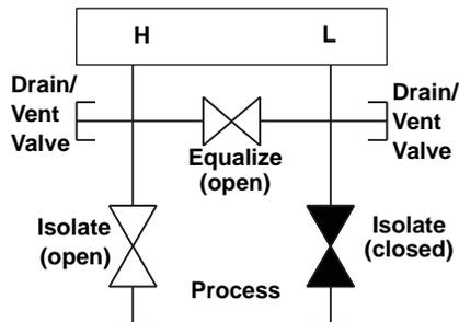
3. After zeroing the transmitter, close the equalizing valve.
