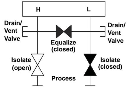
4. Open the block valve on the low pressure side of the transmitter to return the transmitter to service.
