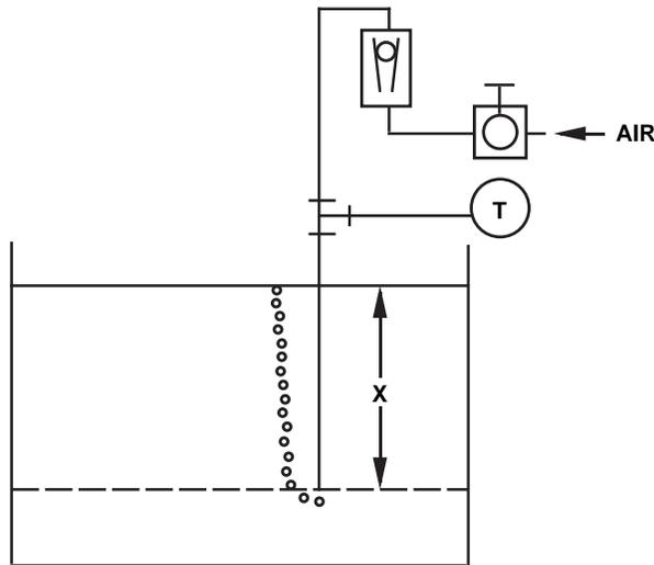
Let **X** equal the vertical distance between the minimum and maximum measurable levels (100 in.).
