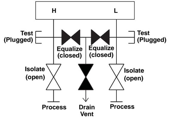
1. To zero the 3051, first close the block valve on the low pressure (downstream) side of the transmitter.
