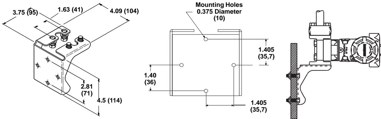
Figure 3-6. Flat Mounting Bracket Option Codes B3 and BC
