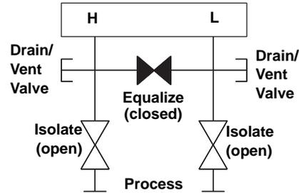
1. To zero the 3051, close the block valve to the low pressure (downstream) side of the transmitter first.
