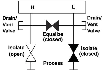
2. Open the center (equalize) valve to equalize the pressure on both sides of the transmitter. The manifold valves are now in the proper configuration for zeroing the transmitter.
