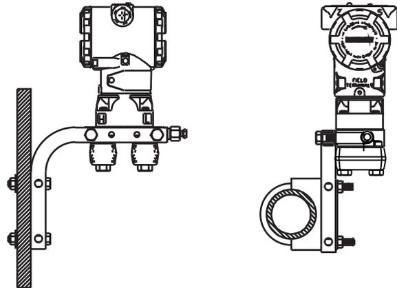
Figure 3-3. Mounting Bracket Option Codes B1, B7, and BA
