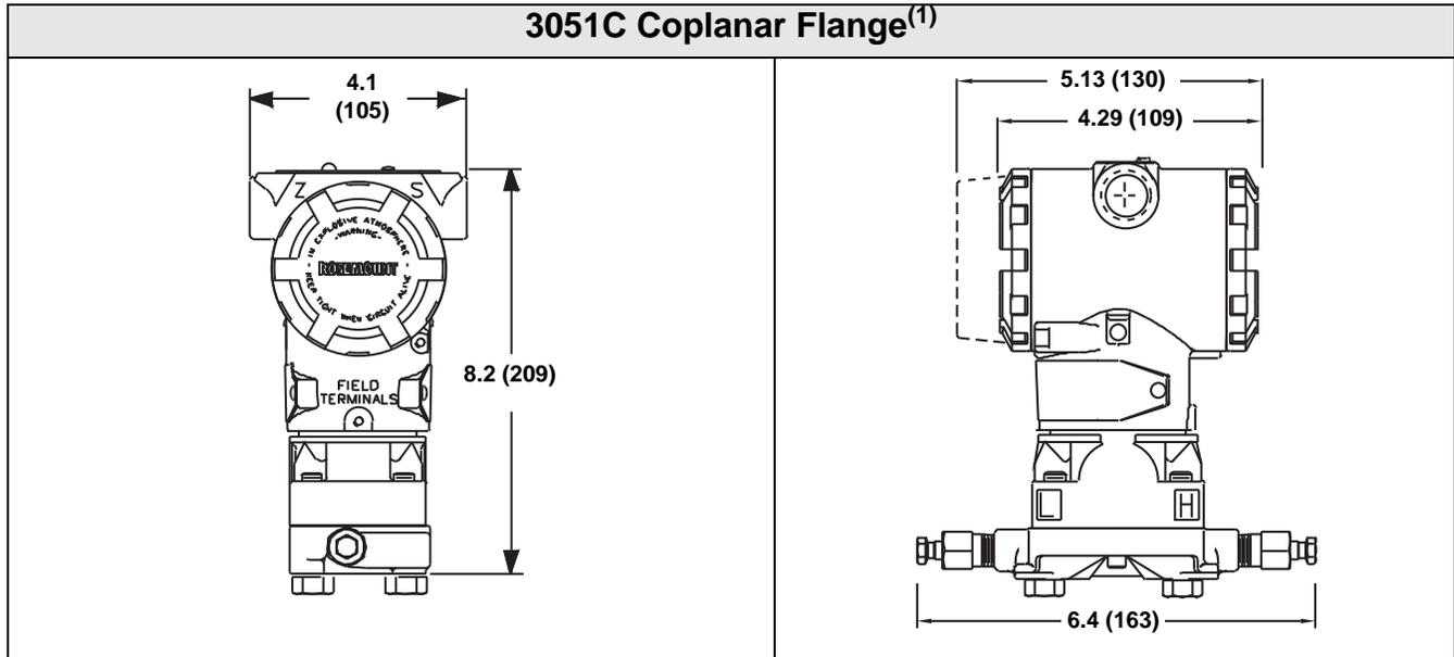
(1) For FOUNDATION fieldbus and Profibus PA transmitters with LCD Display, housing length is 5.36 in. (136 mm).
