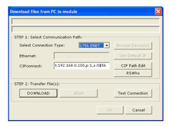
4 Click **RSWHO** to display modules on the network. The MVI56E-MCM module will automatically be identified on the network.
