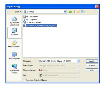
This action opens the **IMPORT CONFIGURATION** dialog box. Click **TAGS** under **MAINROUTINE** to show the controller tags that will be created. Note that if you are using a controller revision number of 16 or less, the **IMPORT CONFIGURATION** dialog box does not show the **IMPORT CONTENT** tree.
