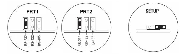
The Setup Jumper acts as "write protection" for the module's firmware. In "write protected" mode, the Setup pins are not connected, and the module's firmware cannot be overwritten. The module is shipped with the Setup jumper OFF. Do not jumper the Setup pins together unless you are directed to do so by ProSoft Technical Support (or you want to update the module firmware).
