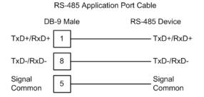
**Note:** Terminating resistors are generally not required on the RS-485 network, unless you are experiencing communication problems that can be attributed to signal echoes or reflections. In these cases, installing a 120-ohm terminating resistor between pins 1 and 8 on the module connector end of the RS-485 line may improve communication quality.
