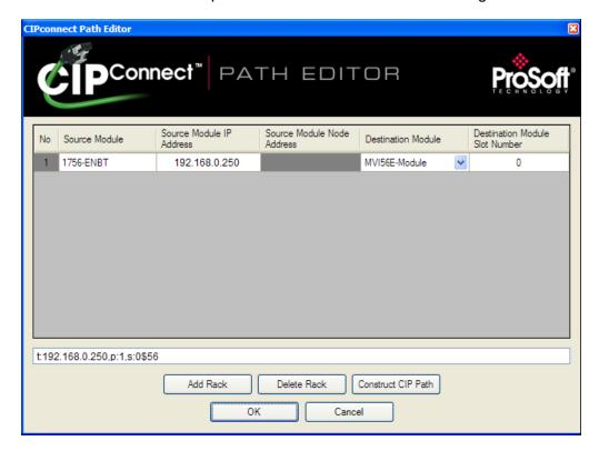
The CIPconnect Path Editor allows you to define the path between the PC and the MVI56E-MCM module. The first connection from the PC is always a 1756-ENBT (Ethernet/IP) module.
