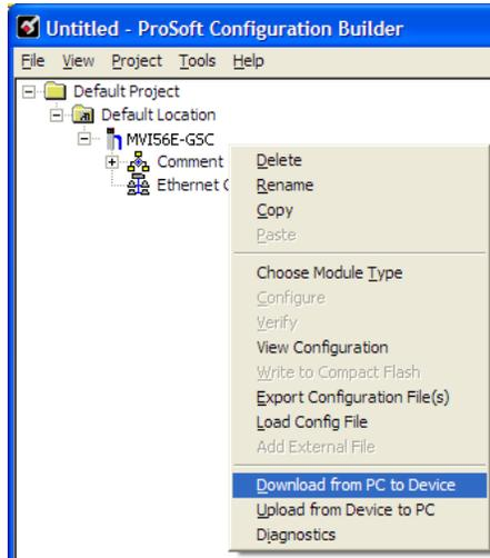
This action opens the **DOWNLOAD** dialog box. Notice that the Ethernet address field contains the temporary IP address you assigned previously. ProSoft Configuration Builder will use this temporary IP address to connect to the module.
