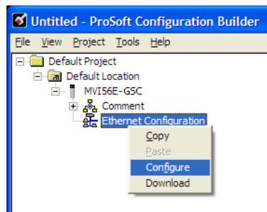
This action opens the *Edit-WATTCP* dialog box. Use this dialog box to enter the MVI56E-GSC module's permanent IP Address (**MY\_IP**), **SUBNET MASK (NETMASK)** and **DEFAULT GATEWAY (GATEWAY)**.
