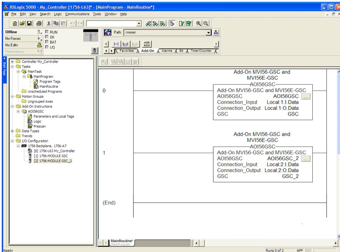
The setup procedure is now complete. Save the project and download the application to your ControlLogix processor.
