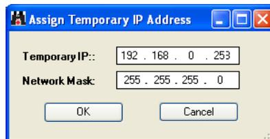
**Important:** The temporary IP address is only valid until the next time the module is initialized. For information on how to set the module's permanent IP address, see *Setting Up a Permanent IP Address* (page 22).
