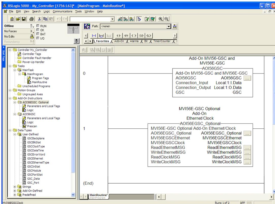
You will notice that new tags have been imported: four **MESSAGE** tags: **WRITEETHERNETMSG**, **WRITECLOCK.MSG**, **READCLOCKMSG**, and **READETHERNETMSG** tags.
