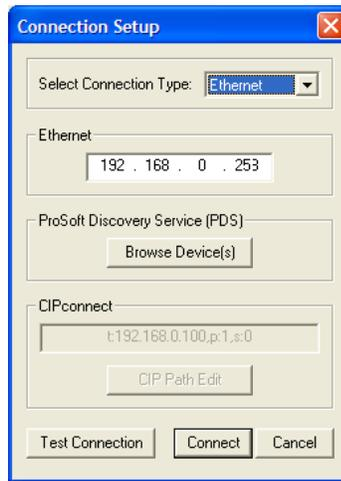
You can also use CIPconnect® to connect to the module through a 1756-ENBT card. Refer to *Using CIPconnect® to Connect to the Module* (page 25) for information on how to construct a CIP path.
