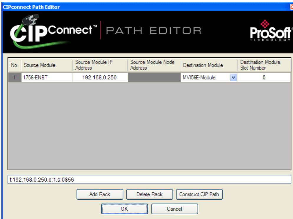
The *CIPconnect Path Editor* allows you to define the path between the PC and the MVI56E-GSC module. The first connection from the PC is always a 1756-ENBT (Ethernet/IP) module.
