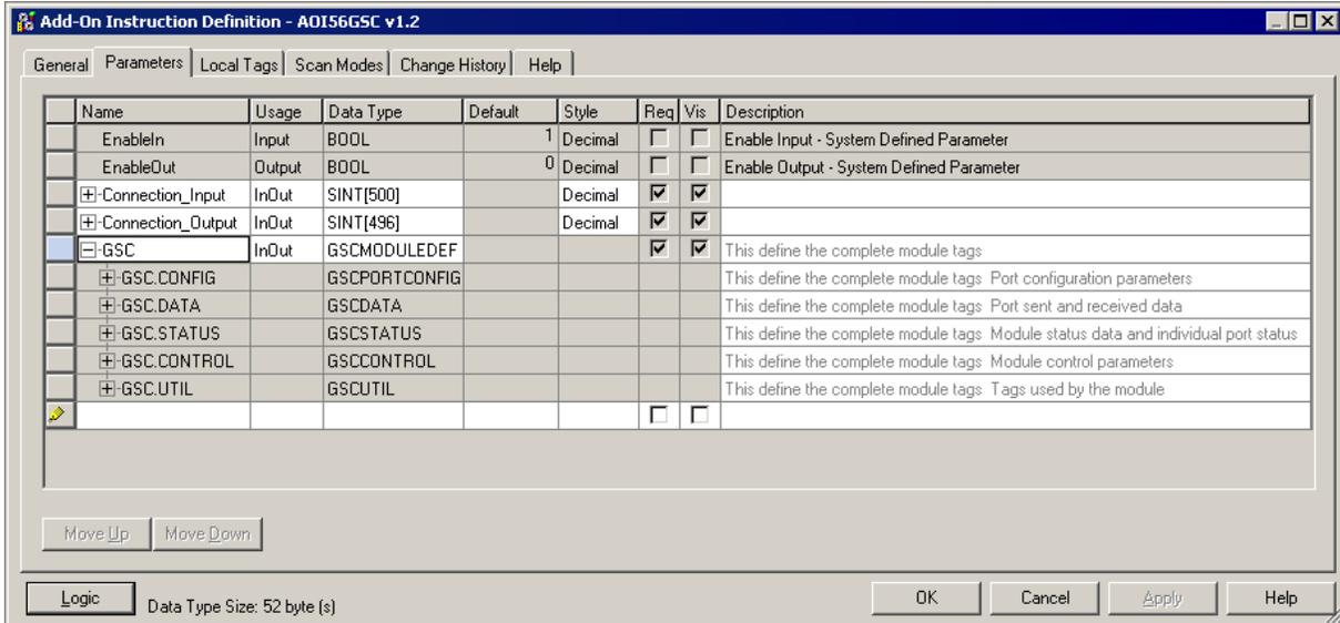
The **ENABLEIN** and **ENABLEOUT** Boolean tags allow you to enable or disable input to or output from the AOI to the rest of the program. For normal operation, these two tags must be set to a value of one (1). Setting either tag or both tags to zero (0) will cause loss of communication and backplane transfer errors.
