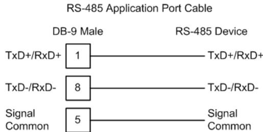
**Note:** Terminating resistors are generally not required on the RS-485 network, unless you are experiencing communication problems that can be attributed to signal echoes or reflections. In these cases, installing a 120-ohm terminating resistor between pins 1 and 8 on the module connector end of the RS-485 line may improve communication quality.
