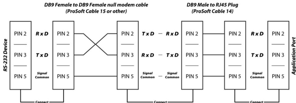
RS-232: Modem Connection (Hardware Handshaking Required)
