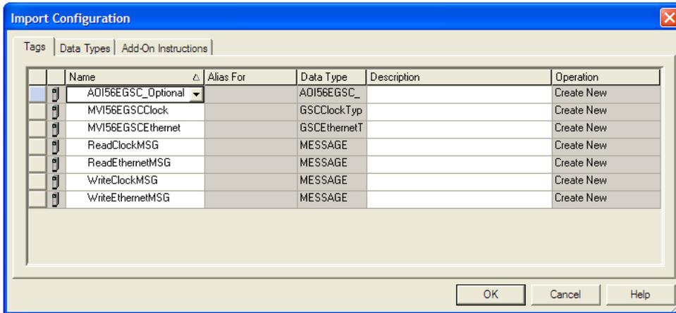
The Optional Add-On Instruction will be now visible in the ladder logic. Observe that the procedure has also imported data types and controller tags associated to the Optional Add-On Instruction.
