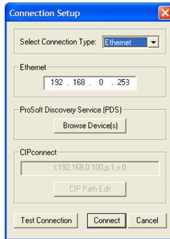
You can also use CIPconnect<sup>®</sup> to connect to the module through a 1756-ENBT card. Refer to *Using CIPconnect to Connect to the Module* (page 64) for information on how to construct a CIP path.
