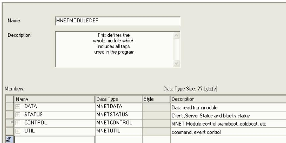
Click the **[+]** signs to expand the UDT structures and view lower-level UDTs.
