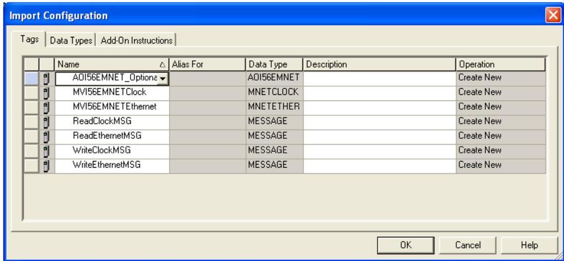
The Optional Add-On Instruction will now be visible in the ladder logic. Observe that the procedure has also imported data types and controller tags associated with the Optional Add-On Instruction.
