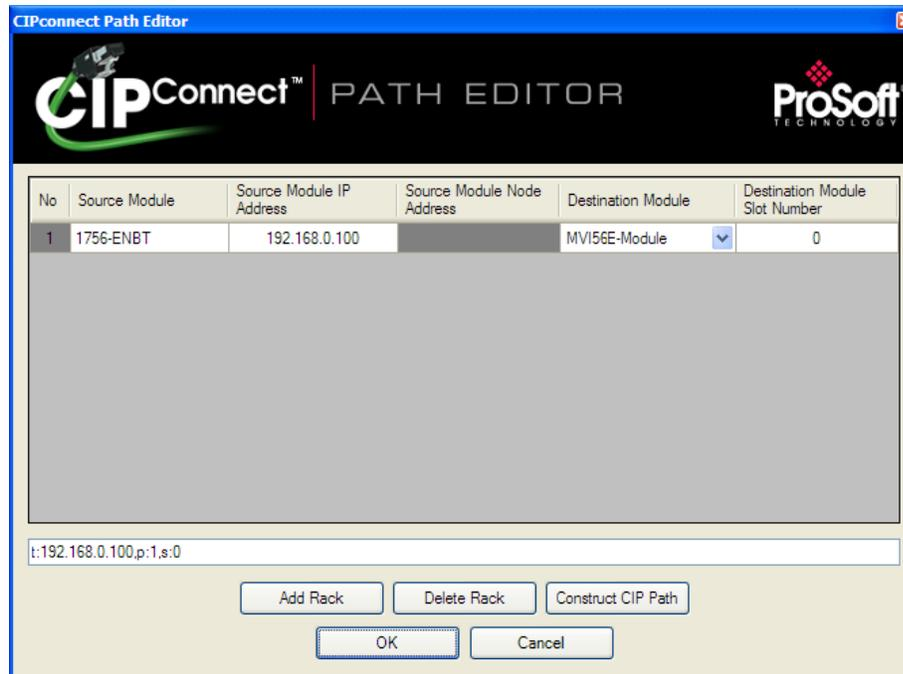
The *CIPconnect Path Editor* allows you to define the path between the PC and the MVI56E-MNET module. The first connection from the PC is always a 1756-ENBT (Ethernet/IP) module.
