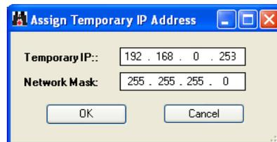
**Important:** The temporary IP address is only valid until the next time the module is initialized. For information on how to set the module's permanent IP address, see Ethernet Configuration (page 58).
