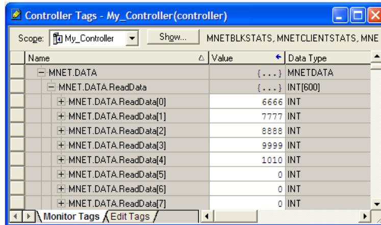
The *ReadData* array is related to the contents of the Read Data area of the module's internal database. To view the actual registers in the module's internal database, access the database display from *ProSoft Configuration Builder's Diagnostics* menu. For more information, see the section on *PCB Diagnostics* (page 96).
