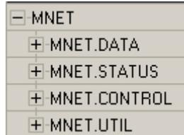
The four lower-level controller tag structures contain other controller tags and controller tag structures. Click the **[+]** sign next to any controller tag structure to expand it and view the next level in the structure.
