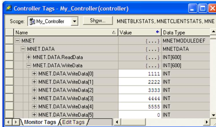
The *WriteData* array is related to the contents of the Write Data area of the module's internal database. To view the actual registers in the module's internal database, access the database display from *ProSoft Configuration Builder's Diagnostics* menu. For more information, see the section on *PCB Diagnostics* (page 96).
