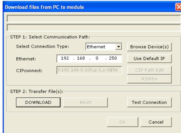
Click **TEST CONNECTION** to verify that the IP address allows access to the module.
