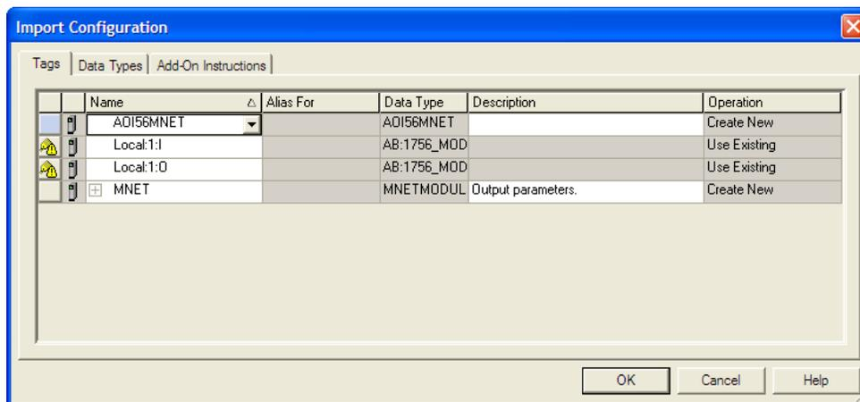
11 Associate the I/O connection variables to the correct module. The default values are **LOCAL:1:I** and **LOCAL:1:O** so these require change.
