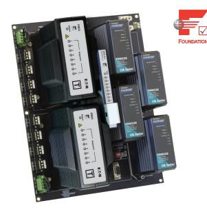
FF-831 validation test for power conditioners. There is also galvanic isolation between the fieldbus segments, thereby preventing multiple segment failures from ground faults on more than one segment. Each segment has its own fieldbus power conditioner and current limitation. Termination of the fieldbus segment is automatically maintained when single or redundant F80x modules are fitted.
