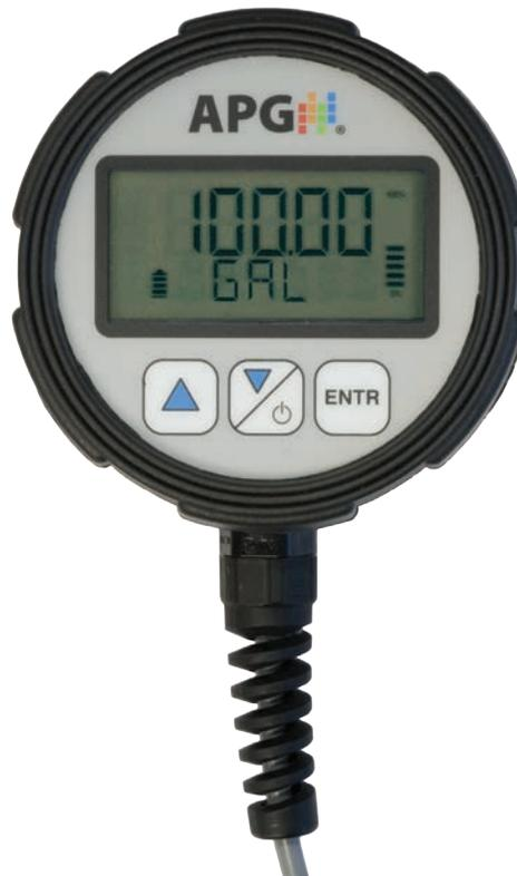
The MND Modbus Network Display provides a local display that can be wired to a local Tank Cloud network, or modbus sensor, displaying readings from any of the sensors in the network (up to ten). It is easy to use and very flexible. The MND can operate in either a master or sniffer mode. With the ability to listen in on sensors or poll sensors for current readings, the MND provides a valuable display option for your network.
