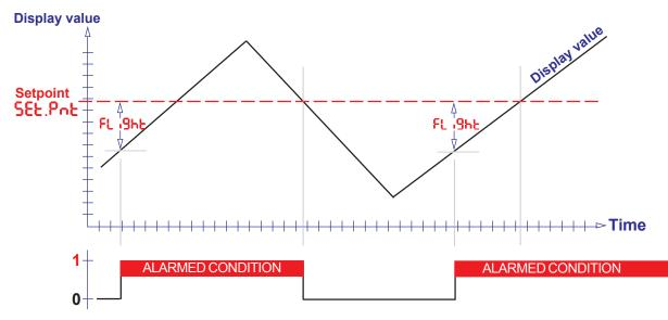
The Setpoint can be placed anywhere you like, in the range **-199999** to **+999999** and will include a decimal point in the appropriate position if you have set your display range to have a decimal point.
