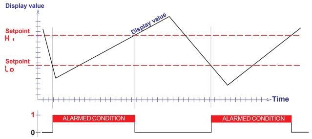
The Setpoints can be placed anywhere you like, in the range -999999 to +9999999 and will include a decimal point in the appropriate position if you have set your display range to have a decimal point.
