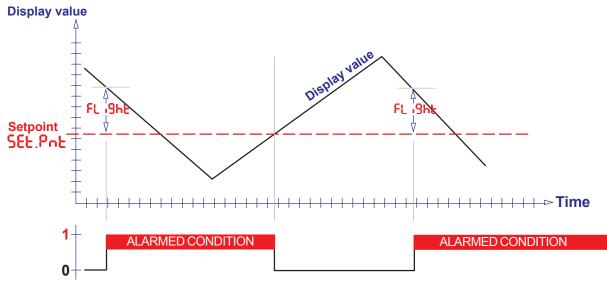
The Setpoint can be placed anywhere you like, in the range **+999999** to **+9999999** and will include a decimal point in the appropriate position if you have set your display range to have a decimal point.
