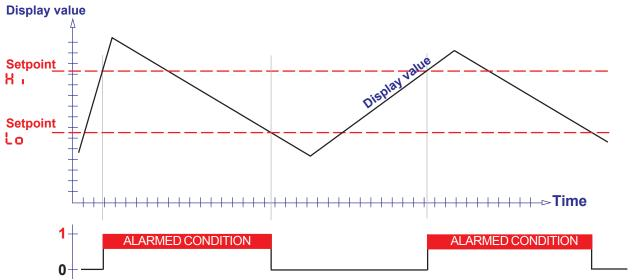
The Setpoints can be placed anywhere you like, in the range **-199999** to **+999999** and will include a decimal point in the appropriate position if you have set your display range to have a decimal point.
