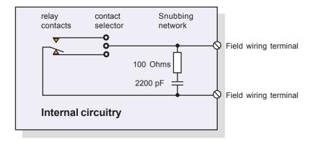
But because you are switching an AC signal, the capacitor is acting as a charge coupler, and your voltmeter is detecting the coupled AC voltage. If you were to use a traditional, lower impedance moving pointer meter, such as an AVO, you would probably not see this effect. The impedance of the capacitor is very high, around 1 500 000 Ohms with 50Hz AC or 1 200 000 Ohms with 60Hz AC.
