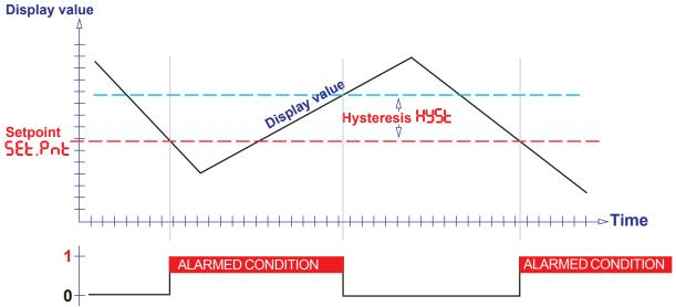
The Setpoint can be placed anywhere you like, in the range **-199999** to **+999999** and will include a decimal point in the appropriate position if you have set your display range to have a decimal point.
