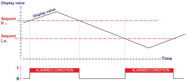
The Setpoints can be placed anywhere you like, in the range **-199999** to **+999999** and will include a decimal point in the appropriate position if you have set your display range to have a decimal point.
