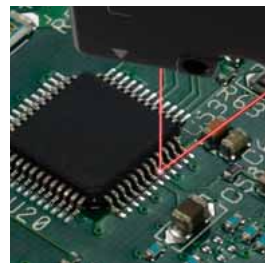
Measurement of the IC pin height
