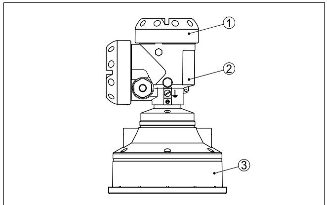
Fig. 1: OPTISOUND 3030 C with Alu double chamber housing
