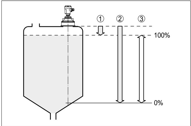
Fig. 3: Min. distance to the max. level
