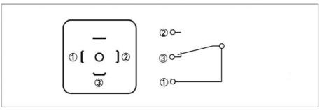
Figure 4-2: Connection of 3-wire reed contact
