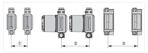
Figure 2-1: Minimum distances when installing several measuring devices
