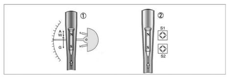
Figure 1-1: Functional principle
