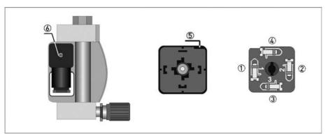
Figure 4-1: Electrical connection of the limit switches (5) Lift slot
