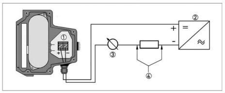
Figure 4-5: Electrical connection M8E
