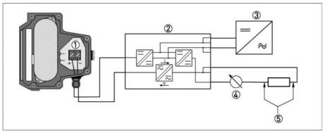
Figure 4-6: Electrical connection with galvanic isolation
