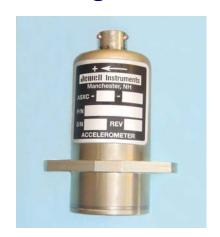
The Jewell ASXC Series Fluid Rotor Angular Accelerometer is a force balance servo accelerometer that uses a fluid-filled ring chamber to measure angular acceleration. The ASXC is currently used in a wide variety of applications including many military and aviation flight controls including autopilot or aircraft stability and control systems or satellite stability.
