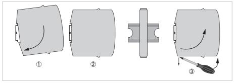
Figure 3-3: Rail installation
