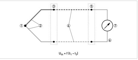
Figure 7-2: Thermocouple measuring circuit, schematic.
