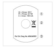
Figure 2-2: Example for bottom nameplate
