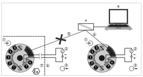
Figure 5-1: Connection during configuration of in-head transmitter
