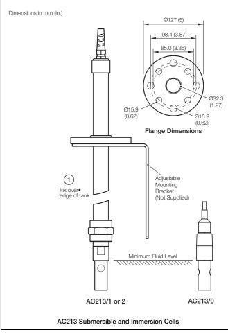
Caution. After cleaning and installing the conductivity cell, ensure that it remains filled with liquid and is not allowed to dry out. Ensure that the electrode bore remains fully immersed at minimum fluid levels.
