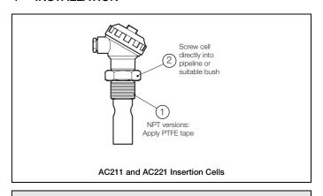
Caution. Overtightening may damage the cell body.
