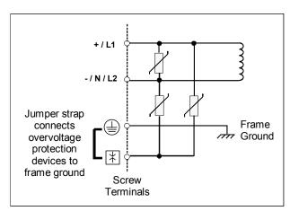
In systems with a floating neutral input (the neutral line is not referenced to Protective Earth Ground), this jumper must NOT be installed. In a floating neutral system, voltage surge protection devices such as MOVs **must** be installed from L1 to earth ground, and from L2 (Neutral) to earth ground.
