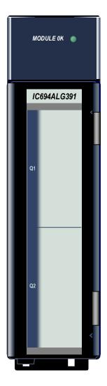
The **2–Channel Analog Current Output** module, IC694ALG391, has two output channels, each capable of converting 12 bits of binary (digital) data to an analog output signal for field devices. Each output can be set using a jumper on the module to produce output signals in one of two ranges:
