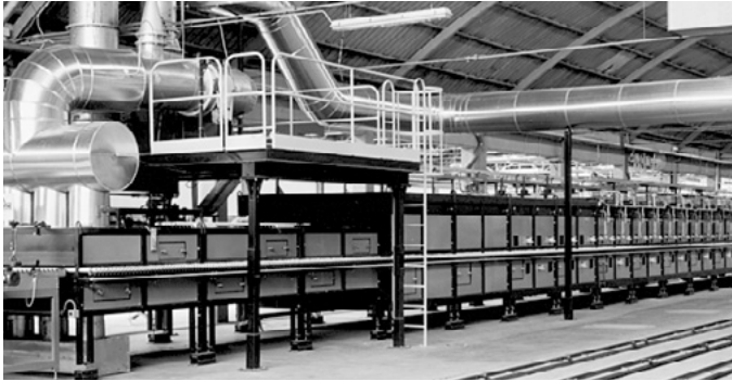
Roller hearth kiln in the ceramics industry
