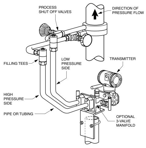
Figure 19. Example of Vertical Process Line Installation
