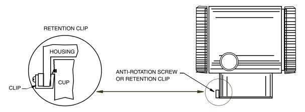
Figure 20. Housing Screw or Clip Location
