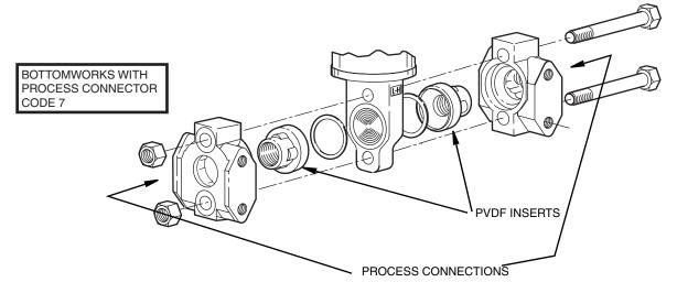
Figure 37. Replacing the Sensor Assembly (pvdf Inserts)
