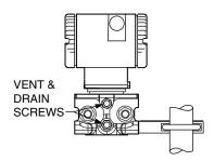
Figure 17. Cavity Venting and Draining
