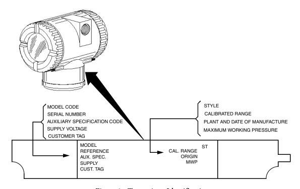
Figure 1. Transmitter Identification
