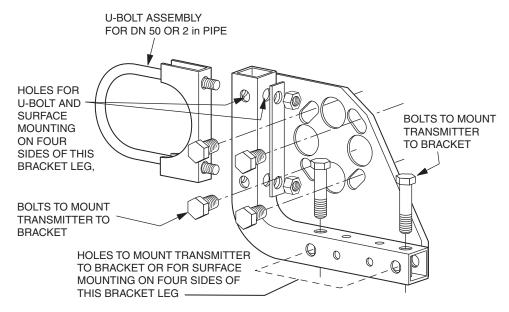
Figure 8. Details of a Universal Bracket
