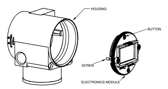
Figure 21. Positioning Display
