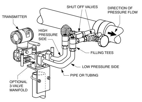
Figure 18. Example of Horizontal Process Line Installation
