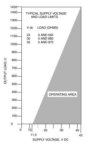
Figure 25. Supply Voltage and Loop Load
