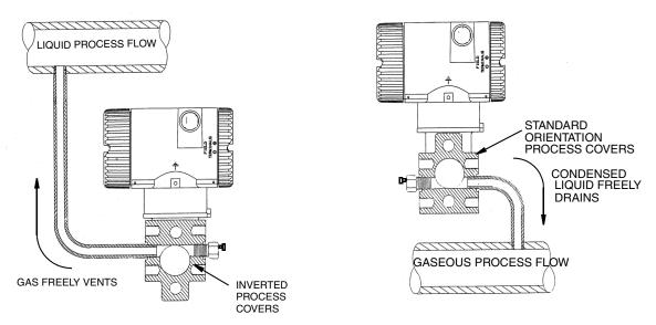
Figure 38. Sensor Cavity Venting and Draining
