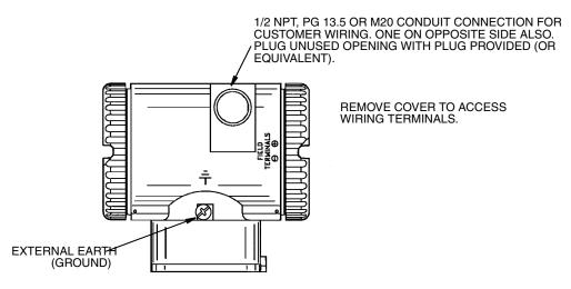
Figure 23. Accessing Field Terminals
