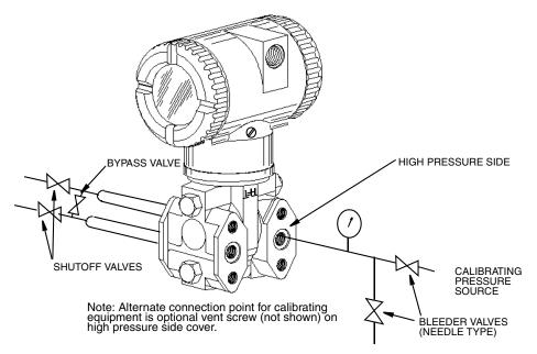
Figure 32. Field Calibration Setup
