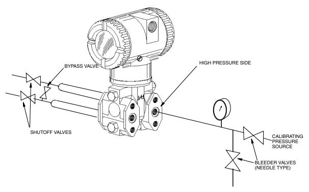
Figure 33. Bench Calibration Setup
