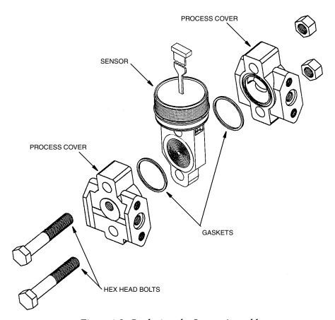
Figure 36. Replacing the Sensor Assembly
