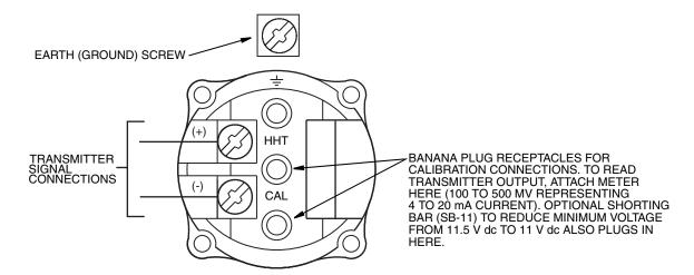
Figure 24. Identification of Field Terminals
