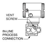
Figure 15. Vertical Mounting - Cavity Venting
