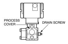
Figure 12. Vertical Mounting - Cavity Draining
