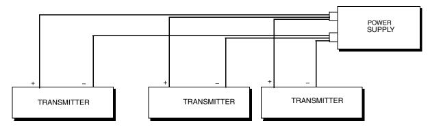
Figure 27. Wiring Several Transmitters to a Common Power Supply
