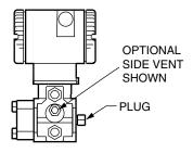
Figure 13. Vertical Mounting - Cavity Venting
