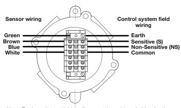
Note: Earth equipotential bonding must be achieved either by the sensor's integral earth conductor or via the sensor rear mounting thread
