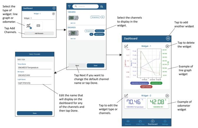
Measurements are updated every second when the logger is within range. Note that measurements displayed in the dashboard may differ from logged data points, which are recorded at the logging interval selected when configuring the logger. When a logger is out of range, the graph widget will not display any measurements and the odometer widget will display the most recent measurement from when the logger last communicated with the phone, tablet, or computer.
