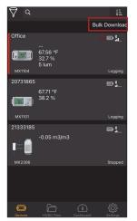
2. The screen changes to Bulk Download mode. This changes the way the screen behaves when you tap on a logger tile. Tap on a tile to select it for Bulk Download. You can select up to 20 loggers. Text at the bottom of the page updates to indicate how many loggers are selected.
