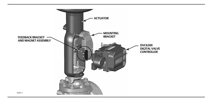
Pneumatic tubing connected to the DVC6200 brings instrument supply air to the DVC6200 and takes controlled output air from the DVC6200 to the actuator. Pressure sensors in the DVC6200 measure these pressure signals and present them as device variables
