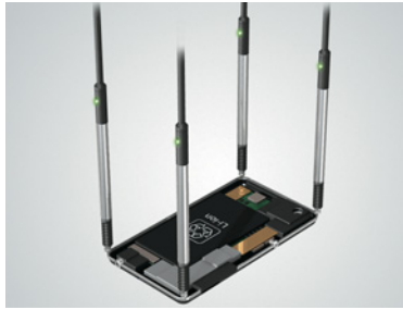
Smartphone chassis flatness inspection
