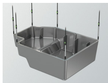
Oil pan flatness measurement
