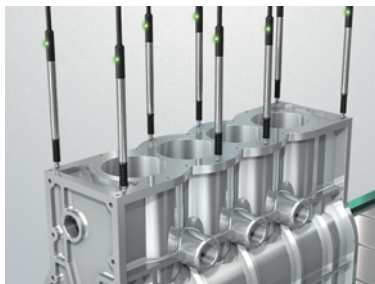
Flatness measurement of engine block
