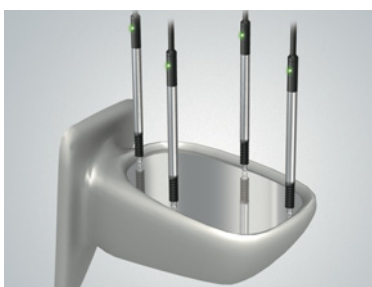
Side mirror angle inspection
