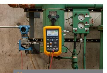
The automatic pump on the 729 pressure calibrator reduces hand pump instrument error as well as reducing calibration time by about 40 %."
