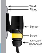
Determine the mounting location for the level switch. The point of actuation (where the sensor will send a "wet" signal) is most often
