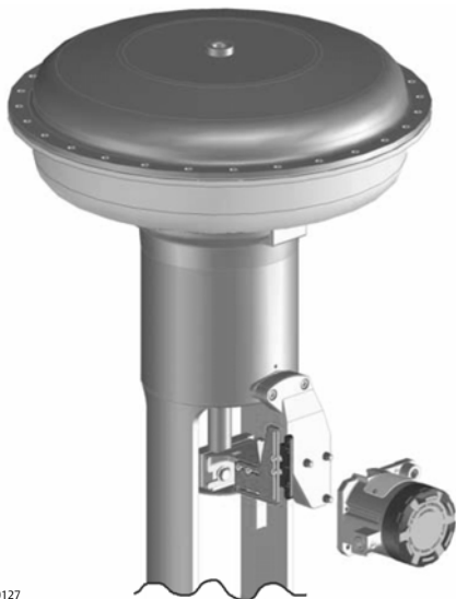
Figure 2-9. Mounting Parts for Sliding-Stem Actuator with up to 210 mm (8.25 Inches) Travel
