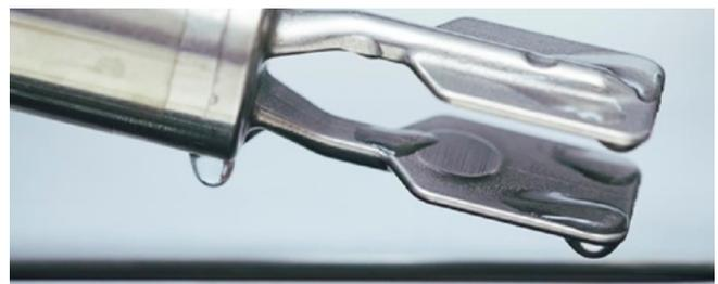
**Figure 2:** The oscillation of a tuning fork instrument changes when a liquid reaches the two forks.
