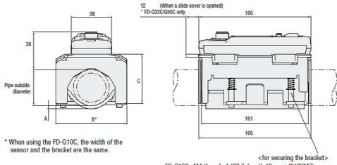
FD-Q10C: M4 thread x4 (P0.7, length 13 mm, SUSXM7) FD-Q20C: M4 thread x4 (P0.7, length 19 mm, SUSXM7) FD-Q32C: M5 thread x4 (P0.8, length 30 mm, SUSXM7) FD-Q50C: M5 thread x4 (P0.8, length 38 mm, SUSXM7)
