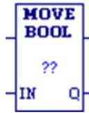
When the MOVE function receives power flow, it copies data as individual bits from one location in PLC memory to another. Because the data is copied in bit format, the new location does not need to be the same data type as the original.
