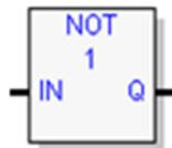
The Logical Not or Logical Invert (NOT) function sets the state of each bit in the output bit string Q to the opposite of the state of the corresponding bit in bit string IN1.
