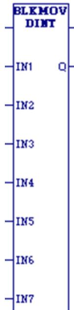
When the Block Move (BLKMOV) function receives power flow, it copies a block of seven constants into consecutive locations beginning at the destination specified in output Q. BLKMOV passes power to the right whenever it receives power.
