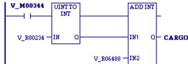
Whenever input %M00344 is set, the UINT value in %R00234 is converted to a signed integer (INT) and passed to the ADD function, where it is added to the INT value in %R06488. The sum is output by the ADD function to the reference CARGO.
