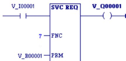
When the enabling input %I0001 is ON, SVC\_REQ function number 7 is called, with the parameter block starting at %R0001. If the operation succeeds, output coil %Q0001 is set ON.
