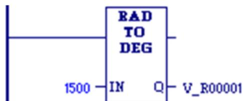
A value of +1500 radians is converted to degrees. The result is placed in %R00001 and %R00002.
