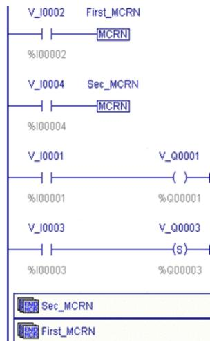
The example at right an MCRN named Sec\_MCRN nested inside the MCRN named First\_MCRN. Whenever the V\_I0002 contact allows power flow into the MCRN function, program execution will continue without power flow to the coils until the associated ENDMCRN is reached. If the V\_I0001 and V\_I0003 contacts are ON, the V\_Q0001 coil is turned OFF and the SET coil V\_Q0003 maintains its current state.
