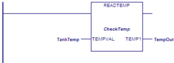
The function block ReadTemp contains the following logic, which uses an ARG\_PRES function to determine whether a value for TempVal is present. If TempVal does not have a value, Temp\_Pres is OFF and Idle is ON. If a value exists for TempVal, the ARG\_PRES function sets Temp\_Pres ON. When Temp\_Pres and Switch are both ON, Start is set ON.
