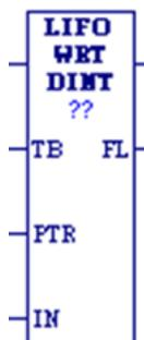
The Last-In-First-Out (LIFO) Write (LIFO\_WRT) function increments the table pointer by one and then adds an entry at the new pointer location in a table. Values are always moved in at the top of the table. If the pointer reaches the last location and the table becomes full, LIFO\_WRT cannot add further values. LIFO\_RD must then be used to remove the entry at the pointer location and decrement the pointer by one.
