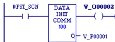
On the first scan (as restricted by the #FST\_SCN system variable), a command block consisting of 100 words of data, including the 6 header words, is copied to %P00001 through %P00100. %Q00002 receives power.
