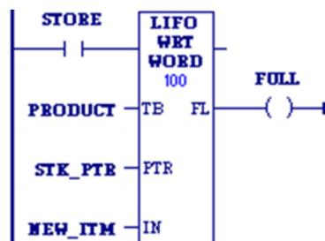
PRODUCT is a LIFO table with 100 word-sized elements. When the enabling input STORE is ON, a data item from NEW\_ITEM is copied to the table location pointed to by the value in STK\_PTR. Output FL passes power when PTR = LEN, firing the FULL coil. No further data from NEW\_ITEM can be added to the table without first copying data out, using the LIFO\_RD function.
