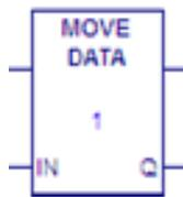
The MOVE\_DATA function copies the variable assigned to the input, IN to the variable assigned to the output, Q. If the constant 0 is assigned to IN, the variable assigned to Q is initialized to its default value.
