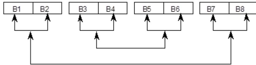
Character (ASCII) strings or BCD data require no adjustment since the Intel and Motorola conventions for storage of character strings are identical.
