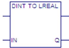
When DINT\_TO\_LREAL receives power flow, it converts the double-precision input data to 64-bit double-precision floating point data.
