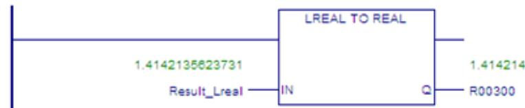
The double-precision floating point value of the square root of 2 is rounded to the nearest single-precision floating point value and placed in R00300.
