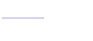
Horizontal and vertical wires (H\_WIRE and V\_WIRE) are used to connect elements of a line of LD logic between functions. Their purpose is to complete the flow of logic (power) from left to right in a line of logic.
