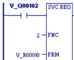
When %Q00102 is set, the CPU places the current time values of the windows in the parameter block starting at location %R0010.
