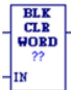
When the Block Clear (BLKCLR\_WORD) function receives power flow, it fills the specified block of data with zeroes, beginning at the reference specified by IN. When the data to be cleared is from BOOL (discrete) memory (%I, %Q, %M, %G, or %T), the transition information associated with the references is updated. BLKCLR\_WORD passes power to the right whenever it receives power.
