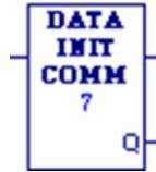
The Data Initialize Communications Request (DATA\_INIT\_COMM) function initializes a COMMREQ function with a block of constant data. The IN parameter of the COMMREQ must correspond with output Q of this DATA\_INIT\_COMM function.
