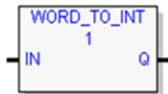
Converts the input data into the equivalent single-precision signed integer (INT) value, which it outputs to Q. This function does not change the original input data. The output data can be used directly as input for another program function, as in the examples.
