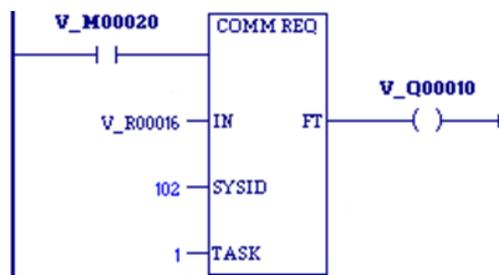
When enabling input %M0020 is ON, a command block starting at %R0016 is sent to communications task 1 in the device located at rack 1, slot 2 of the PLC. If an error occurs processing the COMMREQ, %Q0100 is set.
