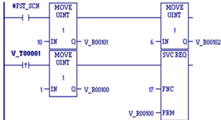
When %T00001 transitions on, alarm interrupts from input %AI0006 are masked. The parameter block at %R00100 is set up on the first scan.
