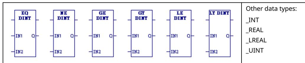
When the relational function receives power flow, it compares input IN1 to input IN2. These operands must be the same data type. If inputs IN1 and IN2 are equal, the function passes power to the right, unless IN1 and/or IN2 is NaN (Not a Number). The following relational functions can be used to compare two numbers:
