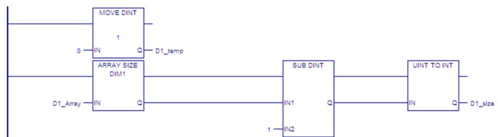
In the following rungs, the FOR\_LOOP executes when D1ON is set to On. The variable index D1\_Index increments by 1 from 0 through D1\_size, the value calculated by ARRAY\_SIZE\_DIM1 and SUB\_DINT. In each loop, the value of D1\_temp is assigned to the element D1\_Array[D1\_Index] and D1\_temp is increased by 1.
