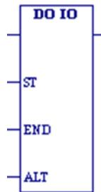
When the DO I/O (DO\_IO) function receives power flow, it updates inputs or outputs for one scan while the program is running. You can also use DO\_IO to update selected I/O during the program in addition to the normal I/O scan.
