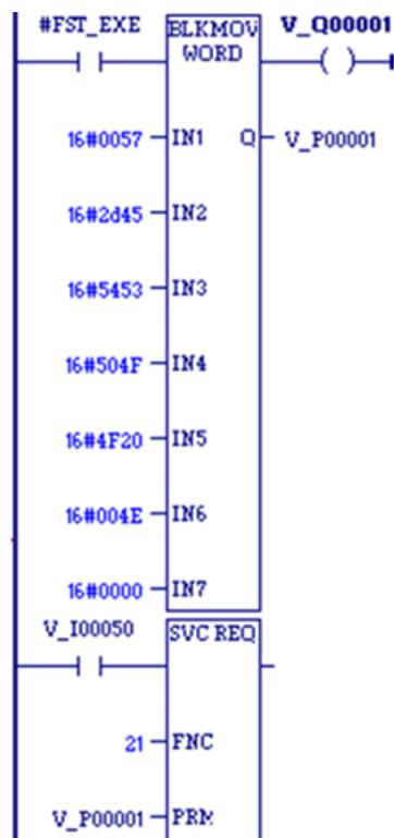
The value passed to IN1 is the fault error code. The value passed in, 16x0057, represents an error code of 87 decimal and will appear as part of the fault message. The values of the next inputs give the ASCII codes for the text of the error message.
