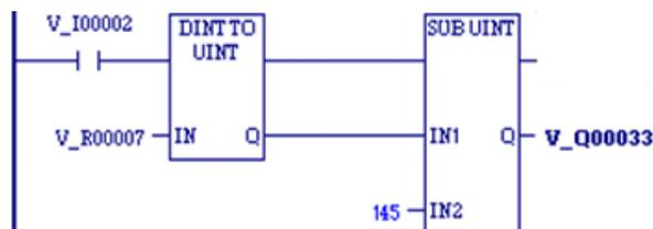
Whenever input %I00002 is set and no errors exist, the double precision signed integer (DINT) at input location %R00007 is converted to an unsigned integer (UINT) and passed to the SUB function, where the constant value 145 is subtracted from it. The result of the subtraction is stored in the output reference location %Q00033.
