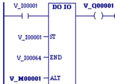
When DO\_IO receives power flow, the PLC scans references %I0001—64 and %Q0001 is turned on. A copy of the scanned inputs is placed in internal memory from %M0001-64. Because a reference is specified for ALT, the real inputs are not updated. This allows the current values of inputs to be compared with their values at the beginning of the scan. This form of DO\_IO allows input points to be scanned one or more times during the program execution portion of the CPU scan.
