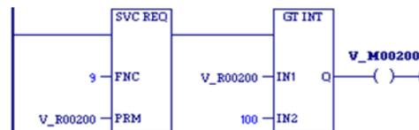
**Note:** Higher resolution (in nanoseconds) can be obtained by using SVC\_REQ 51: Read Sweep Time from Beginning of Sweep.
