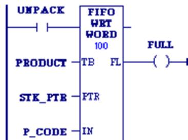
PRODUCT is a FIFO table with 100 word-sized elements. When the enabling input UNPACK is ON, a data item from P\_CODE is copied to the table location pointed to by the value in STK\_PTR. Output node FL passes power when PTR = LEN, firing the FULL coil. No further data from P\_CODE can be added to the table without first copying data out, using the FIFO\_RD function.
