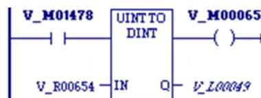
Whenever input %M01478 is set, the unsigned single-precision integer (UINT) value at input location %R00654 is converted to a double-precision signed integer (DINT) and the result is placed in location %L00049. The output %M00065 is set whenever the function executes successfully.
