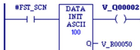
On the first scan (as restricted by the #FST\_SCN system variable) the decimal equivalent of 100 bytes of ASCII text is copied to %R00050 through %R00149. %Q00002 receives power.
