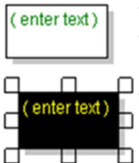
The Text block is used to place an explanation in the program. When you type in a comment, the first few words are displayed.
