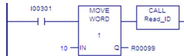
When enabling input %I0301 goes ON, register location %R0099 is loaded with the value 10, which is the function code for the Read Target Name function. The program block READ\_ID is then called to retrieve the target name. The parameter block is located at address %R0100.
