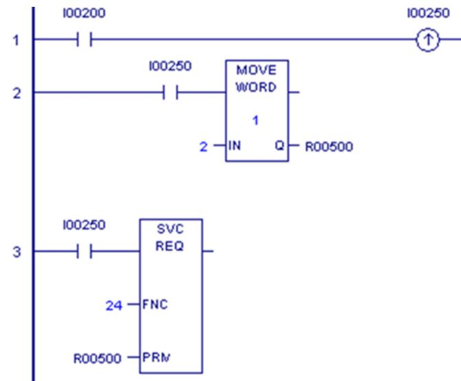
This example resets the module in rack0/slot 2.
