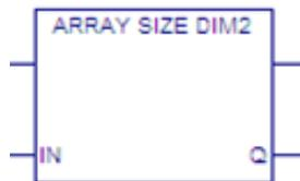
Returns the value of the Array Dimension 2 property of an array and writes the value to output Q. If a non-array variable is assigned to IN, the value of Q is 0.
