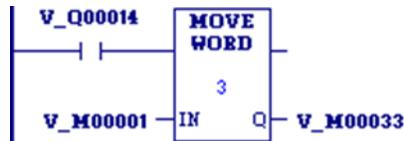
V\_M00001 and V\_M00033 are both WORD arrays of length 3, for a total of 48 bits in each array. Since PLCs do not recognize arrays, Length must be set at 3, for the total number of WORDs to be moved. When enabling input V\_Q0014 is ON, MOVE\_WORD moves 48 bits from the memory location %M00001 to memory location %M00033. Even though the destination overlaps the source for 16 bits, the move is done correctly.
