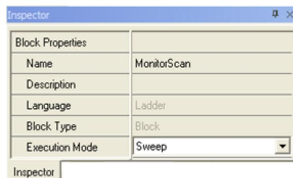
4. Go online to the Controller and select Programmer Mode. Put the Controller in RUN Mode or STOP Enabled Mode.
