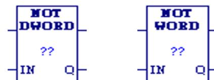
When the Logical Not or Logical Invert (NOT) function receives power flow, it sets the state of each bit in the output bit string Q to the opposite of the state of the corresponding bit in bit string IN1.
