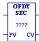
The Off-Delay Timer (OFDT) increments while power flow is off, and the timer's Current Value (CV) resets to zero when power flow is on. OFDT passes power until the specified interval PV (Preset Value) has elapsed.
