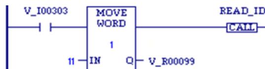
When enabling input %I0303 is ON, register location %R0099 is loaded with the value 11, which is the function code for the Read Controller ID function. The program block READ\_ID is then called to retrieve the ID. The parameter block is located at address %R0100.
