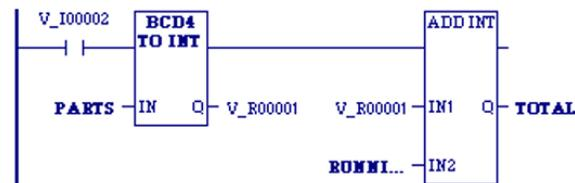
Whenever input %I0002 is set, the BCD-4 value in PARTS is converted to a signed integer (INT) and passed to the ADD\_INT function, where it is added to the INT value represented by the reference RUNNING. The sum is output by ADD\_INT to the reference TOTAL.
