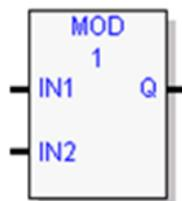
Divides input IN1 by input IN2 and outputs the remainder of the division to Q.
