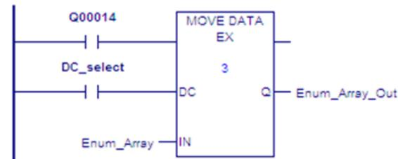
Enum\_Array and Enum\_Array\_Out are arrays of enumerated variables, with three elements each. To copy all elements in Enum\_Array, input Length should be 3. When the enabling input Q00014 is on, MOVE\_DATA\_EX copies three elements from memory location Enum\_Array to memory location Enum\_Array\_Out.
