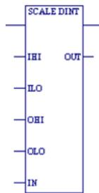
When the SCALE function receives power flow, it scales the input operand IN and places the result in the output variable assigned to output operand OUT. The power flow output is energized when SCALE is performed without Overflow.
