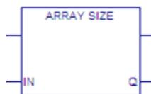
Counts the number of elements in the array assigned to input IN and writes the number to output Q.
