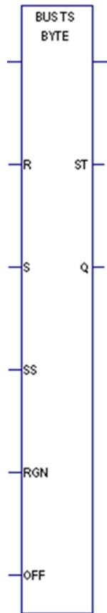
The BUS\_TS function uses semaphores to control access to specific memory in a module located on the bus.
