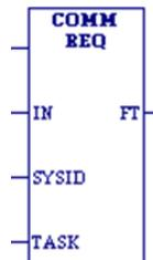
The Communication Request (COMMREQ) function communicates with an intelligent module, such as a Genius Communications Module or High-Speed Counter.
