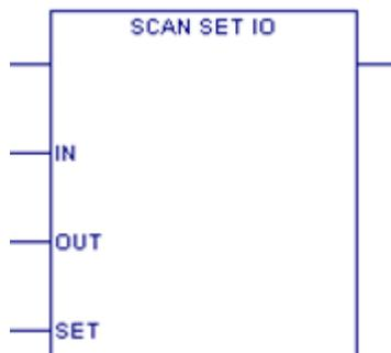
The Scan\_Set\_IO function scans the I/O of a specified scan set number (Modules can be assigned to scan sets in hardware configuration.). You can specify whether the Inputs and/or Outputs of the associated scan set will be scanned.
