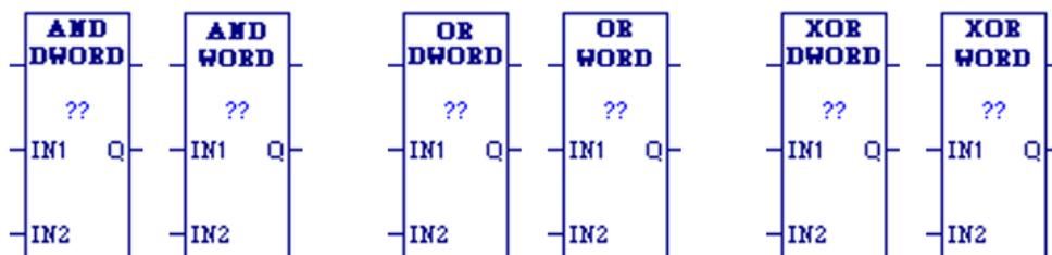
Each scan that power is received, the Logical function examines each bit in bit string IN1 and the corresponding bit in bit string IN2, beginning with the least significant bit in each. You can specify a string length of 1 to 256 WORDS or DWORDS. The IN1 and IN2 bit strings specified may overlap.
