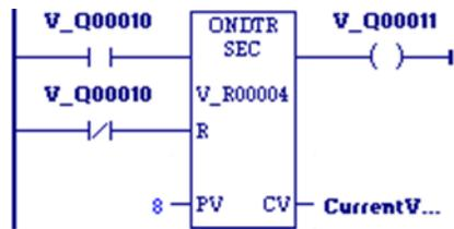
A retentive on-delay timer is used to create a signal (%Q0011) that turns on 8.0 seconds after %Q0010 turns on, and turns off when %Q0010 turns off.
