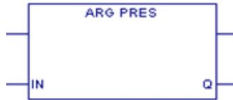
The ARG\_PRES function determines whether an input parameter value was present when the function block instance of the parameter was invoked. This may be necessary if the parameter is optional.
