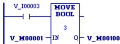
When %I00003 is set, the three bits %M00001, %M00002, and %M00003 are moved to %M00100, %M00101, and %M00102, respectively. Coil %Q00001 is turned on.
