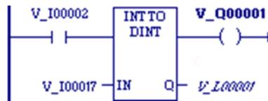
Whenever input %I00002 is set, the signed single-precision integer (INT) value at input location %I00017 is converted to a double-precision signed integer (DINT) and the result is placed in location %L00001. The output %Q01001 is set whenever the function executes successfully.
