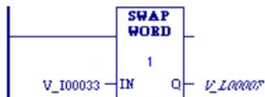
Two bytes located in bits %I00033 through %I00048 are swapped. The result is stored in %L00007.
