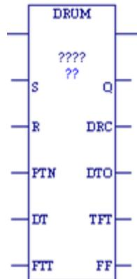
The Drum function operates like a mechanical drum sequencer, which steps through a set of potential output bit patterns and selects one based on inputs to the function. The selected value is copied to a group of 16 discrete output references.
