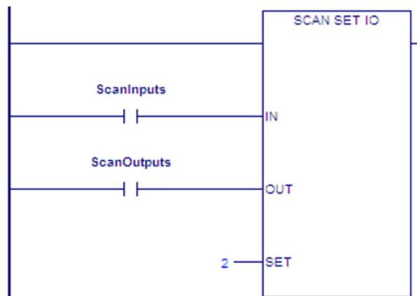
By using the Scan Set IO function block in an interrupt block, you can create a custom I/O scan. For example, two Scan Set IO function blocks can be used in an interrupt block to scan the inputs of a scan set at the beginning of the block and the outputs of the same scan set at the end of the block.
