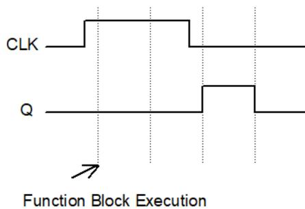
When the CLK input goes from true to false, the output Q is true for one function block instance execution. The output Q then remains false until a new falling edge is detected.
