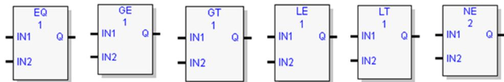
The relational functions compare input IN1 to input IN2. These operands must be the same data type. If inputs IN1 and IN2 are equal, the function outputs the result to Q, unless IN1 and/or IN2 is NaN (Not a Number). The following relational functions can be used to compare two numbers:
