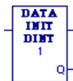
The Data Initialization (DATA\_INIT) function copies a block of constant data to a reference range.
