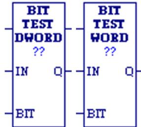
When the Bit Test function receives power flow, it tests a bit within a bit string to determine whether that bit is currently 1 or 0. The result of the test is placed in output Q.
