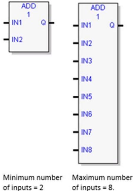
Adds the operands IN1 and IN2 ... IN8 and stores the sum in Q. IN1 ... IN8 and Q must be of the same data type.
