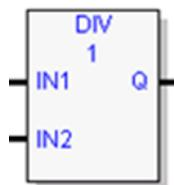
Divides the operand IN1 by the operand IN2 of the same data type as IN1 and stores the quotient in the output variable assigned to Q, also of the same data type as IN1 and IN2.
