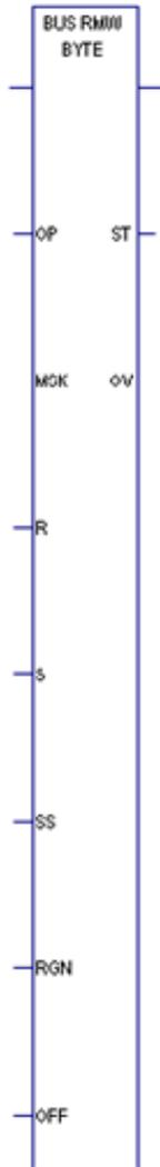
The BUS\_RMW function updates one byte, word, or double word of data on the bus. This function locks the bus while performing the read-modify-write operation.
