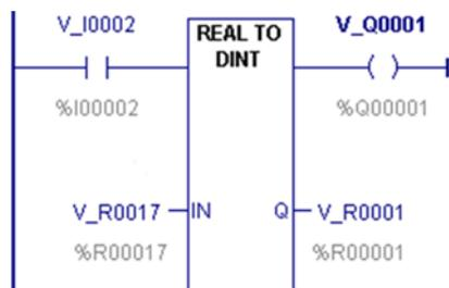
Whenever input %I00002 is set, the REAL value at input location %R00017 is converted to a double precision signed integer (DINT) and the result is placed in location %R00001. The output %Q1001 is set whenever the function executes successfully.
