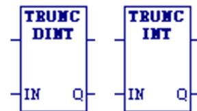
When power is received, the Truncate functions TRUNC\_DINT and TRUNC\_INT round a floating-point (REAL) value down respective to the nearest signed double-precision signed integer (DINT) or signed single-precision integer (INT) value. TRUNC\_DINT and TRUNC\_INT output the converted value to Q. The original data is not changed.
