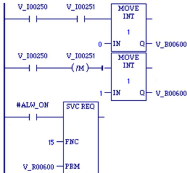
When inputs %I0250 and %I0251 are both on, the first Move function places a zero (read Controller Fault Table) into the parameter block for SVC\_REQ 15. When input %I0250 is on and input %I0251 is off, the Move instruction instead places a one (read I/O Fault Table) in the SVC\_REQ parameter block. The parameter block is located at location %R0600.
