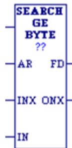
When the Search function receives power, it searches the specified memory block for a value that satisfies the search criteria. For example, SEARCH\_GE\_DWORD searches for a DWORD that is greater than or equal to the specified value (the IN operand).
