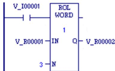
Whenever input V\_I0001 is set, the input bit string in location %R0001 is rotated left 3 bits and the result is placed in %R0002. The actual input bit string %R0001 is left unchanged. If the same reference had been used for IN and Q, a rotation would have occurred in place.
