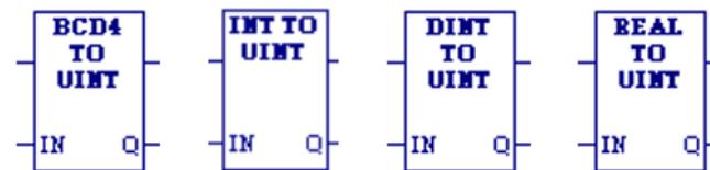
When this function receives power flow, it converts the input data into the equivalent single-precision unsigned integer (UINT) value, which it outputs to Q.
