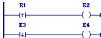
Coil E2 is turned ON when the value of the variable E1 transitions from OFF to ON. It stays ON until E1 is written to again, causing the POSCON to stop passing power flow.
