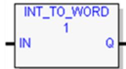
Converts a 16-bit signed integer (INT) operand IN to a 16-bit bit string (WORD) value and stores the result in the variable assigned to Q.
