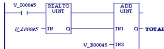
Whenever input %I00045 is set, the REAL value in %L00045 is converted to an unsigned single-precision integer (UINT) and passed to the ADD\_UINT function, where it is added to the UINT value in %R00045. The sum is output by ADD\_UINT to the reference TOTAL.
