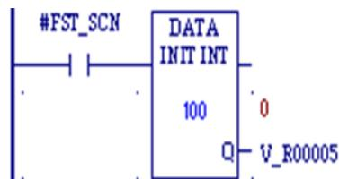
On the first scan (as restricted by the #FST\_SCN system variable), 100 words of initial data are copied to %R00005 through %R00104.
