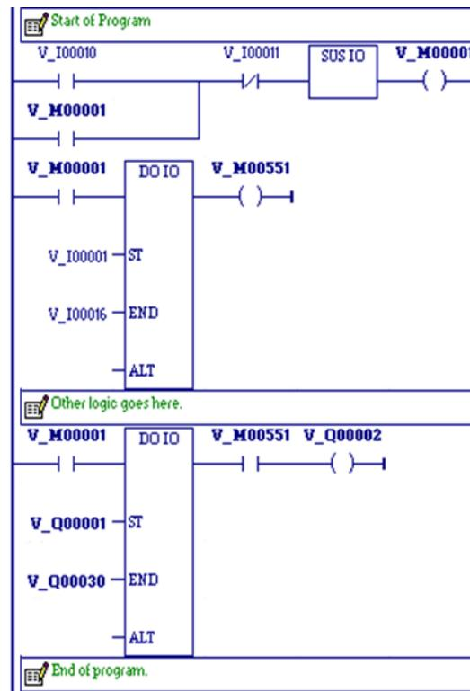
The example at right shows a SUS\_IO function and a DO\_IO function used to stop I/O scans, then cause certain I/O to be scanned from the program.
