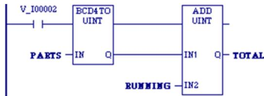
In the example at right, whenever input %I0002 is set, the BCD4 value in PARTS is converted to an unsigned single-precision integer (UINT) and passed to the ADD\_UINT function, where it is added to the UINT value represented by the reference RUNNING. The sum is output by ADD\_UINT to the reference TOTAL.
