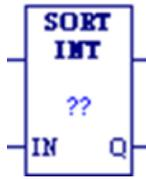
When it receives power flow, the SORT function sorts the elements of the memory block 'IN' in ascending order. The output memory block Q contains integers that give the index that the sorted elements had in the original memory block or list. Q is the same size as IN. It also has a specification (LEN) of the number of elements to be sorted.
