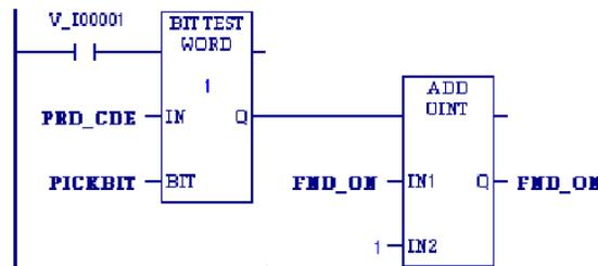
When input V\_I0001 is set, the bit at the location contained in reference PICKBIT is tested. The bit is part of string PRD\_CDE.
