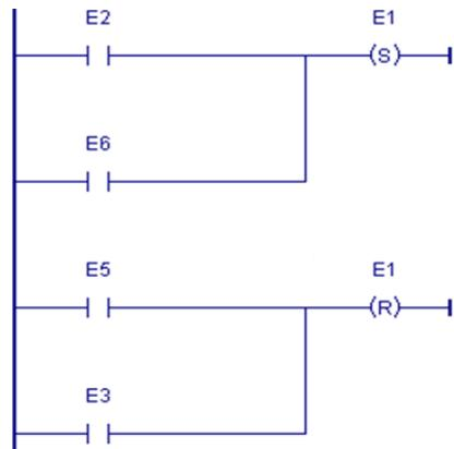
The coil represented by E1 is turned ON when reference E2 or E6 is ON and is turned OFF when reference E5 or E3 is ON
