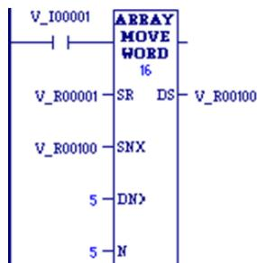
To define the input memory block %R0001 - %R0016 and the output memory block %R0100 - %R0115, SR is set as %R0001, DS is set as %R0100, and Length is set to 16.
