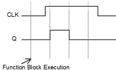
When the CLK input transitions from false to true, the output Q is true for one function block execution. The output Q then remains false until a new rising edge is detected.
