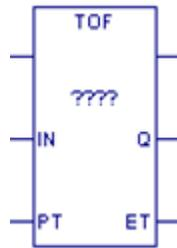
When the input IN transitions from ON to OFF, the timer starts timing until a specified period of time (PT) has elapsed, then sets the output Q to OFF.
