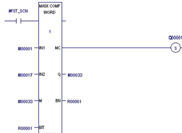
On the first scan, the Masked Compare Word function executes. %M0001 through %M0016 is compared with %M0017 through %M0032. %M0033 through %M0048 contains the mask value. The value in %R0001 determines the bit position in the two input strings where the comparison starts.
