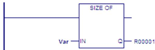
The single-segment structure named Var assigned to input IN contains eight BOOL elements ( $8 \times 1 = 8$  bits) and twelve WORD elements ( $12 \times 16 = 192$  bits). SIZE\_OF outputs the value  $8 + 192 = 200$  to the variable R00001 assigned to output Q.
