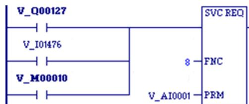
In the LD example at right, power flow through enabling output %Q0127 or input %I1476 or internal coil %M00010 causes the watchdog timer to be reset.
