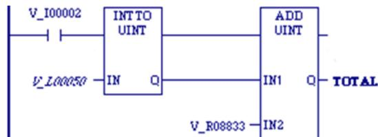
Whenever input %I0002 is set, the INT value in %L00050 is converted to an unsigned single-precision integer (UINT) and passed to the ADD\_UINT function, where it is added to the UINT value in %R08833. The sum is output by ADD\_UINT to the reference TOTAL.
