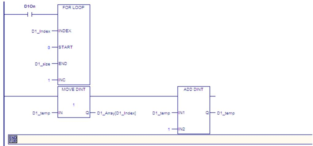
You can use a FOR\_LOOP to iterate through an array's second dimension in a method similar to this example. You can also use nested FOR\_LOOPS to ensure that operations on elements using two variable indexes each do not exceed their array dimension. For additional examples, refer to the online help.
