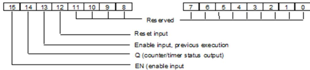
**Note:** Bits 0 through 13 are not used for counters.
