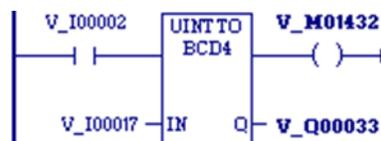
Whenever input %I00002 is set and no errors exist, the UINT at input location %I00017 through %I00032 is converted to four BCD digits and the result is stored in memory locations %Q00033 through %Q00048. Coil %M01432 is used to check for successful conversion.
