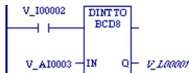
Whenever input %I00002 is set and no errors exist, the double-precision signed integer (DINT) at input location %AI0003 is converted to eight BCD digits and the result is stored in memory locations %L00001 through %L00002.
