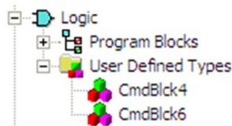
1. In Machine Edition, add a UDT as a node under a target in the Project tab of the Navigator. A UDT will be saved with the target in which it is used.
