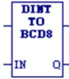
When DINT\_TO\_BCD8 receives power flow, it converts the input signed double-precision integer (DINT) data into the equivalent 8-digit Binary-Coded-Decimal (BCD) values, which it outputs to Q. DINT\_TO\_BCD8 does not change the original DINT data.
