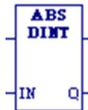
When the function receives power flow, it places the absolute value of input IN into output Q.
