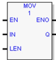
When the input operand, EN, is set to ON, the MOVE instruction copies data as bits from one location in PACSystems controller memory to another. Because the data is copied as bits, the new location does not need to use the same type of memory area as the source. For example, you can copy data from an analog memory area into a discrete memory area, or vice versa.
