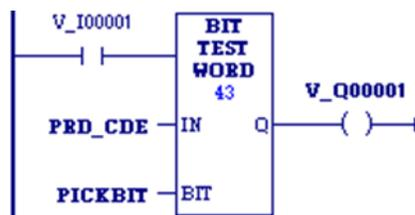
When input V\_I0001 is set, the bit at the location contained in reference PICKBIT is tested. The bit is part of string PRD\_CDE.
