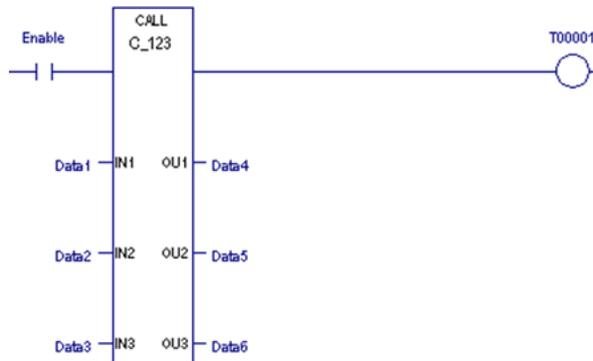
In the example at right, if Enable is set, the C block named C\_123 is executed. C\_123 operates on the input data located at reference addresses Data1, Data2, and Data 3, and produces values located at reference addresses Data4, Data5, and Data6. Logic within C\_123 controls the power flow output.
