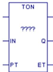
When the input IN transitions from OFF to ON, the timer starts timing until a specified period of time (PT) has elapsed, then sets the output Q to ON.
