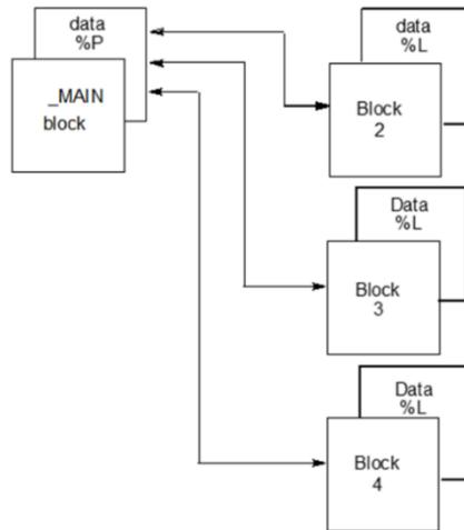
All blocks within the program can use data associated with the `_MAIN` block (`%P`). Blocks and UDFBs can use their own `%L` data as well as the `%P` data that is available to all blocks. The `_MAIN` block cannot use `%L`.
