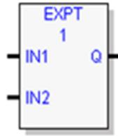
The Power of X (EXPT) function raises the value of input IN1 to the power specified by the value IN2 and places the result in Q. The EXPT function operates on REAL or LREAL input value(s) and place the result in output Q. The instruction is not carried out if one of the following invalid conditions occurs:
