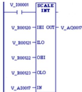
In the example at right, the registers %R0120 through %R0123 are used to store the high and low scaling values. The input value to be scaled is analog input %AI0017. The scaled output data is used to control analog output %AQ0017. The scaling is performed whenever %I0001 is ON.
