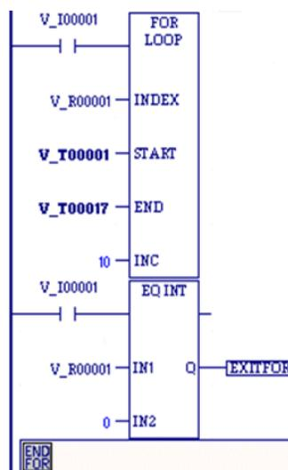
The value for %T00001 (START) is -100 and the value for %T00017 (END) is 100. The INDEX (%R00001) increments by tens, starting at 100 until it reaches its end value of +100. The EQ function of the loop tries to execute 21 times, with the INDEX (%R00001) being equal to 100, -90, -80, -70, -60, -50, -40, -30, -20, -10, 0, 10, 20,
