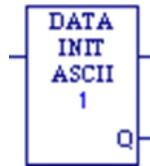
The Data Initialize ASCII (DATA\_INIT\_ASCII) function copies a block of constant ASCII text to a reference range.
