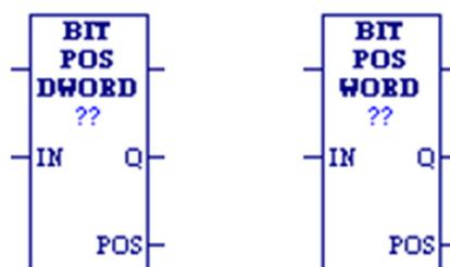
The Bit Position function locates a bit set to 1 in a bit string.
