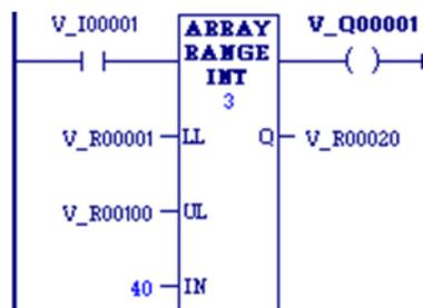
The lower limit (LL) values of %R00001 through %R00008 are 1, 20, 30, 100, 25, 50, 10, and 200. The upper limit (UL) values of %R00100 through %R00108 are 40, 50, 150, 2, 45, 90, 250, and 47. The resulting Q values will be placed in the first 8 bits of %R00200. The bit values low order to high are: 1, 1, 1, 0, 1, 0, 1, and 0. The bit value displayed will be set ON (1) for the low order bit of %R00200. The ok output will be set ON (1).
