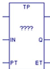
When the input IN transitions from OFF to ON, the timer sets the output Q to ON for the specified time interval, PT has elapsed, then sets the output Q to ON.
