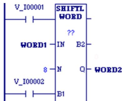
Whenever input V\_I0001 is set, the bits in the input string that begins at WORD1 are copied to the output bit string that starts at WORD2. WORD2 is left-shifted by 8 bits, as specified by the input N. The resulting open bits at the beginning of the output string are set to the value of V\_I0002.
