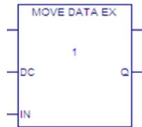
MOVE\_DATA\_EX provides optional data coherency by locking the symbolic memory being written to during the copy operation. This allows data to be copied coherently when accessed by multiple logic threads (i.e. interrupt blocks). Note that copying large amounts of data with coherency enabled can increase interrupt latency.
