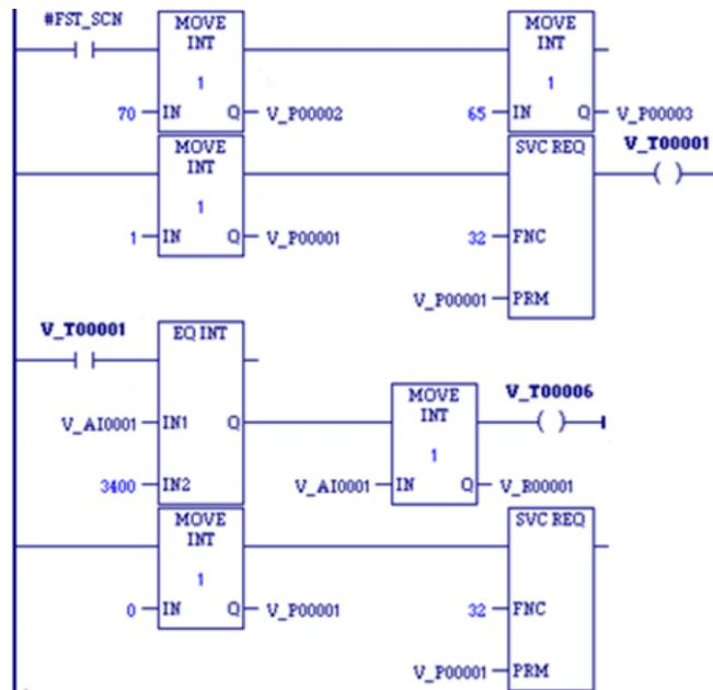
Interrupts from the high-speed counter module whose starting point reference address is %I00065 will be suspended while the CPU solves the logic of the second rung. Without the Suspend, an interrupt from the HSC could occur during execution of the third rung and %T00006 could be set while %R00001 has a value other than 3,400. (%AI0001 is the first non-discrete input reference for the High Speed Counter.)
