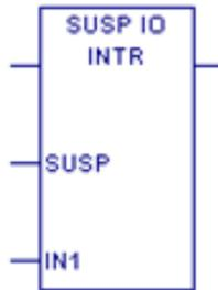
Suspend or resume an I/O interrupt when using I/O variables. If not using I/O variables, use SVC\_REQ 32.
