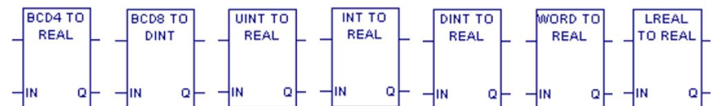
When this function receives power flow, it converts the input data into the equivalent 32-bit floating-point (REAL) value, which its outputs to Q. The conversion to REAL does not change the original input data.
