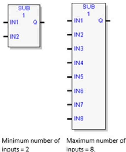
Subtracts the operands IN2 ...IN8 from the operand IN1 and stores the result in the output variable assigned to Q.
