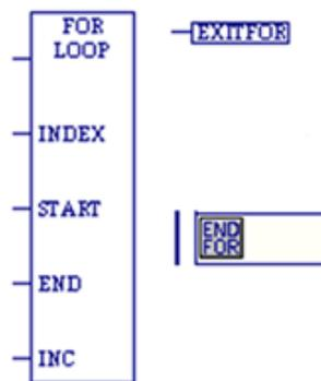
A FOR loop repeats rung logic a specified number of times while varying the value of the INDEX variable in the loop.
