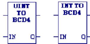
When this function receives power flow, it converts the input unsigned (UINT) or signed single-precision integer (INT) data into the equivalent 4-digit Binary-Coded-Decimal (BCD) values, which it outputs to Q.
