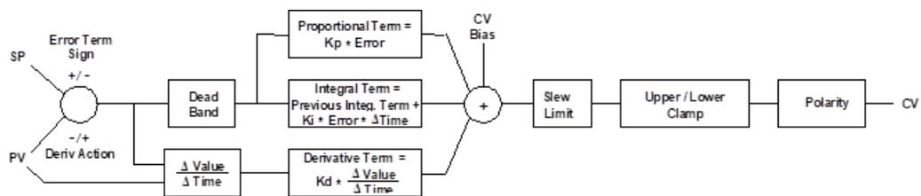
The ISA Algorithm (PID\_ISA) is similar except that its  $K_c$  gain coefficient is applied after the three terms are summed, so that the integral gain is  $K_c / T_i$  and the derivative gain is  $K_c * d$ .
