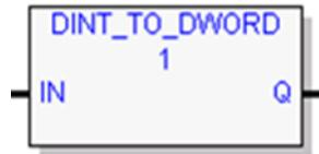
When DINT\_TO\_DWORD receives data, it converts the input double-precision signed integer (DINT) data into the equivalent DWORD (32-bit bit string) value, which it outputs to Q. DINT\_TO\_DWORD does not change the original DINT data.
