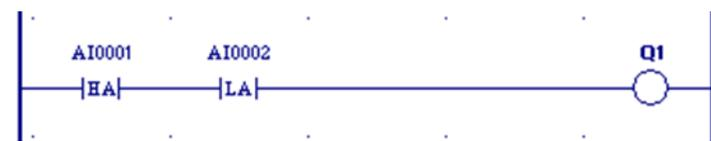
**Note:** HA and LA contacts do not create an entry in a fault table.
