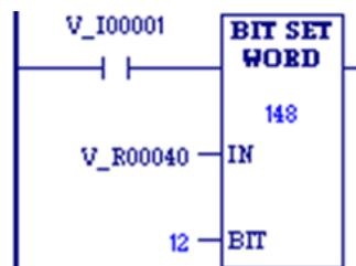
Whenever input V\_I0001 is set, bit 12 of the string beginning at reference %R00040 (as specified by variable V\_R0040) is set to 1.
