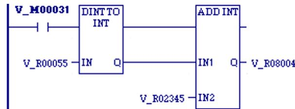
Whenever input %M00031 is set, the DINT value in %R00055 is converted to a signed integer (INT) and passed to the ADD function, where it is added to the INT at %R02345. The sum is output by the ADD function to %R08004.
