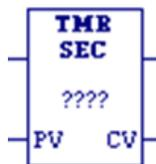
The On-Delay Timer (TMR) increments while it receives power flow and resets to zero when power flow stops. The timer passes power after the specified interval PV (Preset Value) has elapsed, as long as power is received.
