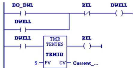
An on-delay timer with address TMRID is used to control the length of time that a coil is on. This coil has been assigned the variable DWELL. When the normally open (momentary) contact DO\_DWL is ON, coil DWELL is energized.
