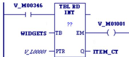
WIDGETS is a table with 20 integer elements. When the enabling input %M00346 is ON, the pointer increments and the contents of the next element of the table are copied into ITEM\_CT. %L00001 functions as the pointer into the data table. %M01001 is used to signal when all items of the data table have been accessed.
