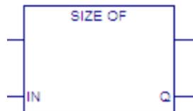
Counts the number of bits used by the variable assigned to input IN and writes the number of bits to output Q. Mnemonics: SIZE\_OF
