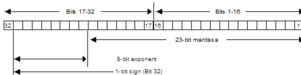
Register use by a single floating-point number is diagrammed below. For example, if the floating-point number occupies registers R5 and R6, R5 is the least significant register and R6 is the most significant register.
