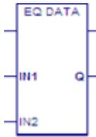
The EQ\_DATA function compares two input variables, IN1 and IN2 of the same data type. If IN1 and IN2 are equal, output Q is energized. If they are not equal, Q is cleared. Mnemonic: EQ\_DATA
