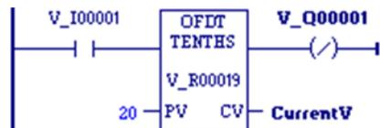
The output action is reversed by the use of a negated output coil. In this circuit, the OFDT timer turns off negated output coil %Q0001 whenever contact %I0001 is closed. After %I0001 opens, %Q0001 stays off for 2 seconds then turns on.
