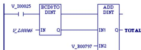
Whenever input %I00025 is set, the BCD-8 value in %L00046 is converted to a signed double-precision integer (DINT) and passed to the ADD\_DINT function, where it is added to the DINT value in %R00797. The sum is output by ADD\_DINT to the reference TOTAL.
