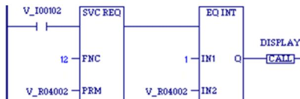
When contact V\_I00102 is ON, the CPU run state is read into location %R4002. If the state is Run/Disabled, the CALL function calls program block DISPLAY.
