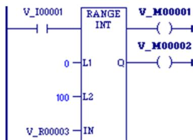
When RANGE\_INT receives power flow from the normally open contact %I0001, it determines whether the value in %R00003 is within the range 0 to 100 inclusively. Output coil %M00002 is ON only if  $0 \leq \%AI0050 \leq 100$ .
