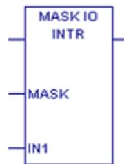
Mask or unmask an interrupt from an I/O board when using I/O variables. If not using I/O variables, use SVC\_REQ 17.
