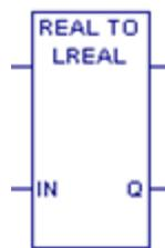
When REAL\_TO\_LREAL receives power flow, it converts the 32-bit single precision floating point REAL data to the equivalent 64-bit double-precision floating point data. REAL\_TO\_LREAL does not change the original REAL data.
