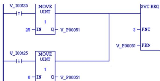
When enabling input %I00125 transitions on, the controller communications window is enabled and assigned a value of 25ms. When the contact transitions off, the window is disabled. The parameter block is in global memory location %P00051.
