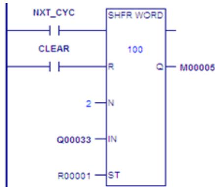
SHFR\_WORD operates on register memory locations %R0001 through %R0100. When the reset reference CLEAR is active, the Shift Register words are set to zero.
