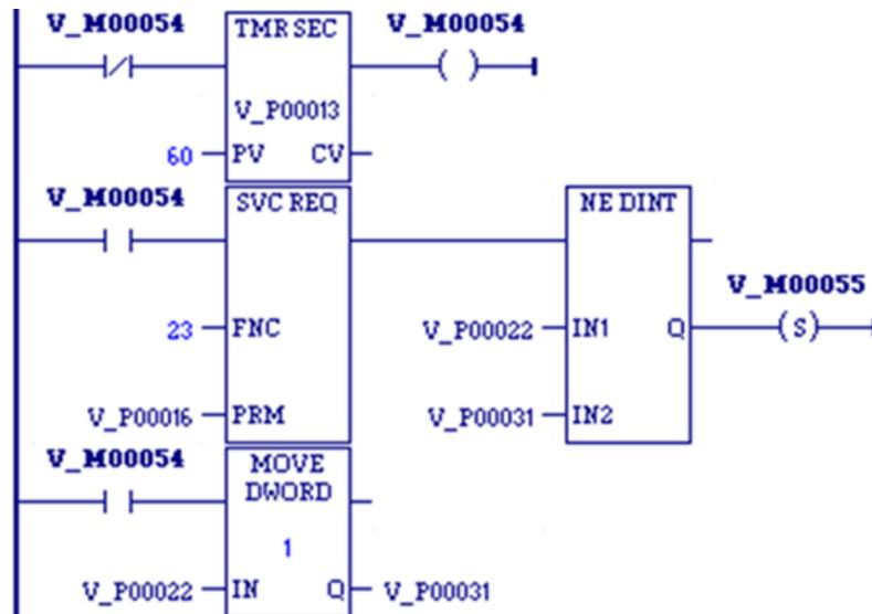
When the timer using registers %P00013 through %P00015 expires, the checksum read is performed. The checksum data returns in registers %P00016 through %P00030. The master program checksum in registers %P00022 and %P00023 (the program checksum is a DWORD data type and occupies two adjacent registers) is compared with the last saved master program checksum. If these are different, coil %M00055 is latched on. The current master program checksum is then saved in registers %P00031 and %P00032.
