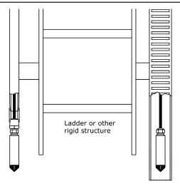
LEVELGAGE, ACCULEVEL or LEVELRAT with optional 1/2"NPT conduit connection. Coupling and conduit provided by customer.
