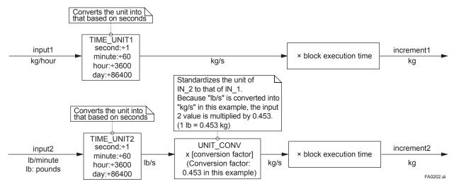
Figure A2.2 Increment Calculation with Rate Input
