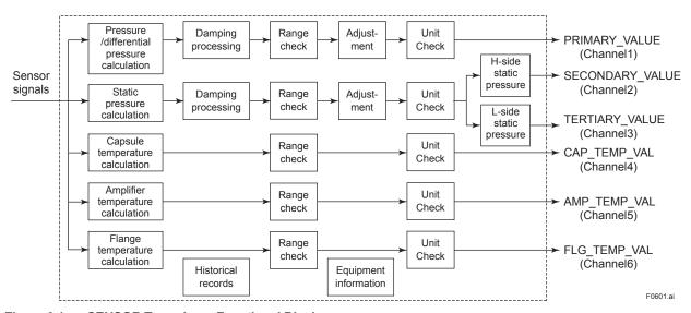
Figure 6.1 SENSOR Transducer Functional Block
