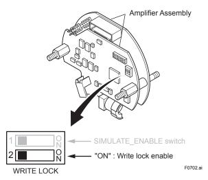
Figure 7.3 Write lock Switch
