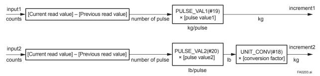
Figure A2.3 Increment Calculation with Counter Input
