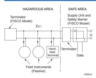
I.S. fieldbus system complying with FISCO model
