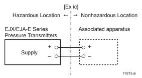
Above drawing shows the installation of entity system. When installing the transmitter in "ic" FISCO system or FNICO system, follow the installation requirements of each system.
