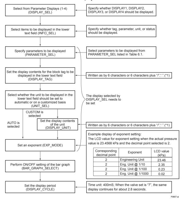
Figure 6.3 Procedures to Set the Built-in Display
