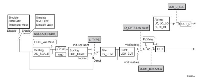
Figure 6.4 Diagram of the Al Functional Block
