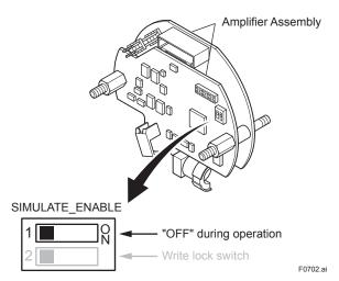
Figure 7.2 SIMULATE\_ENABLE Switch Position
