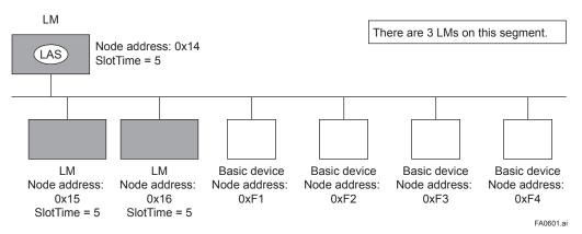
Figure A6.1 Example of Fieldbus configuration-3 LMs on Same Segment
