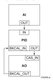
When configuring a simple PID control loop by combining an EJX transmitter with a fieldbus valve positioner that contains an AO block, follow the procedure below to make the settings of the corresponding fieldbus function blocks:
