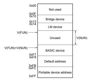
Note 1: Bridge device: A linking device which brings data from one or more H1 networks.
