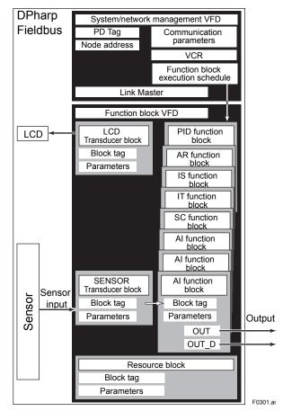
Figure 3.1 Logical Structure of Each Block
