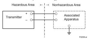
Above drawing shows the installation of Entity system.
