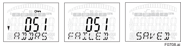
Figure 7.8 Setting screen of Bus Address Configuration
