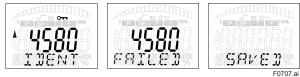
Figure 7.7 Setting screen of Ident Number Configuration
