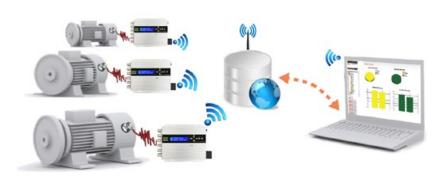
Instruments has created a specific website called EI Analytic that allows the user to remotely access this data and thus determine the condition of the machinery in real time from anywhere in the World. **ERBESSD RELIABILITY**
