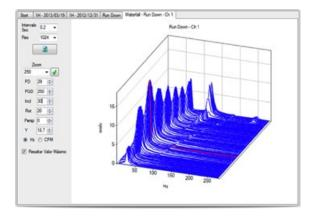
Most spectral tools in DigivibeMX for EIMU are based on the FFT algorithm, capable of measuring low frequencies (1 Hz) up to 10 kHz. The accuracy of the spectrum varies according to the needs, reaching many million of resolution lines.
