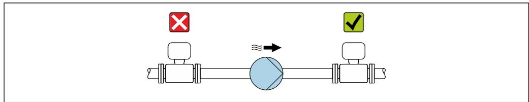
Never install the sensor on the pump suction side in order to avoid the risk of low pressure, and thus damage to the liner.
