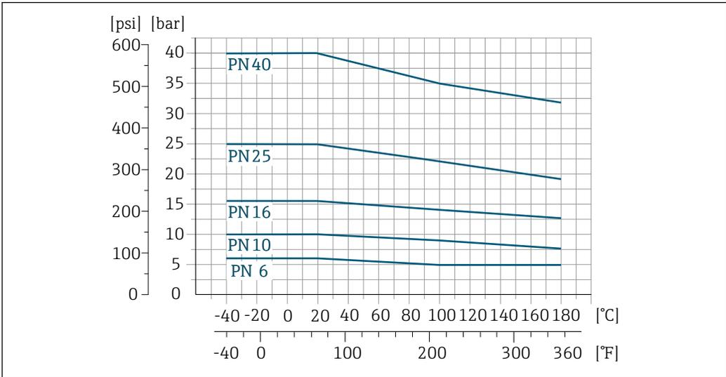
28 Process connection material: stainless steel, 1.4571 (F316L)
