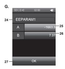
The measurand "water content [ppm]" is a calculated value. For this calculation oil specific parameters (A und B) are needed. The default factory parameter set is [01] EEPARAM1, which contains oil specific parameters for mineral transfomer oil. The determination of other oil-specific parameters can be performed by E+E on request.
