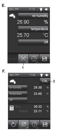
In measurement mode press button (1) in fig. E and select one of the calculation modes shown in fig. B.
