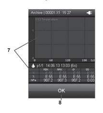
7 Charts (top of fig. C.) and tabulates (bottom of fig. C.) the measured values. You can select one of the three different measurement channels using the "Up" and "Down" keys on the cross control until. The selected measurement channel will be highlighted in the table. Displayed in the table are the minimum value (MIN), the
