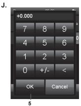
Using the keypad in fig. J, enter the deviation of the current measured value (3) from the reference value.
