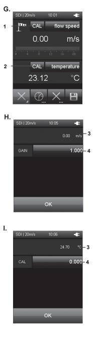
In measurement mode press button CAL (1) or (2) in order to switch to customer adjustment mode (fig. G).
