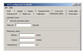
The configuration software allows the EE75 measuring values to be queried periodically on the "Measuring Values" index card.
