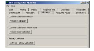
Velocity and temperature calibration is not only possible using the buttons on the integrated display, the EE75 can also easily be calibrated / adjusted using the configuration software.
