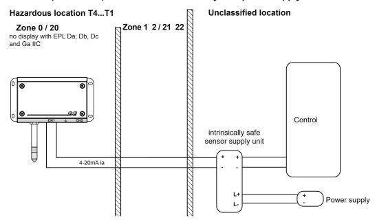
EE300Ex (with remote probe) 2 channels via intrinsically safe power supply device:
