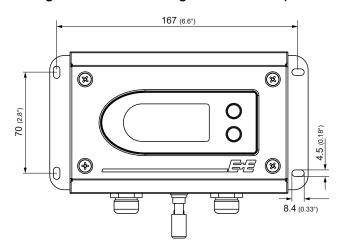
To mount the bottom section use 4 screws diameter < 4.5 mm (0.18")
