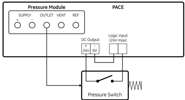
Example Switch Test Connections
