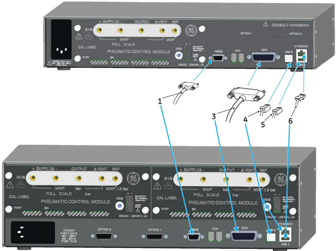
Figure 2-8, Communication Connectors
