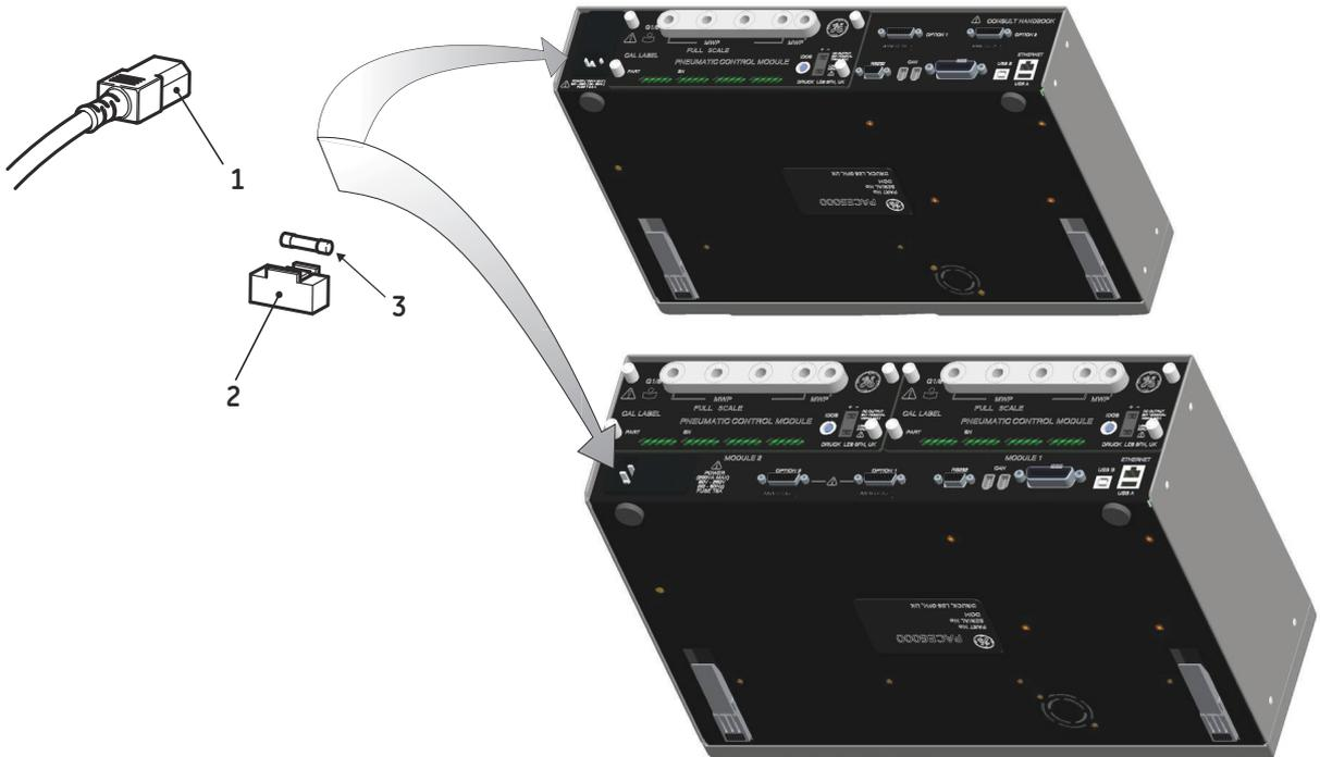
1 - IEC connector    2 - Fuse carrier    3 - Fuse
