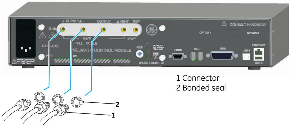
**Figure 2-1, Pneumatic Connections**
