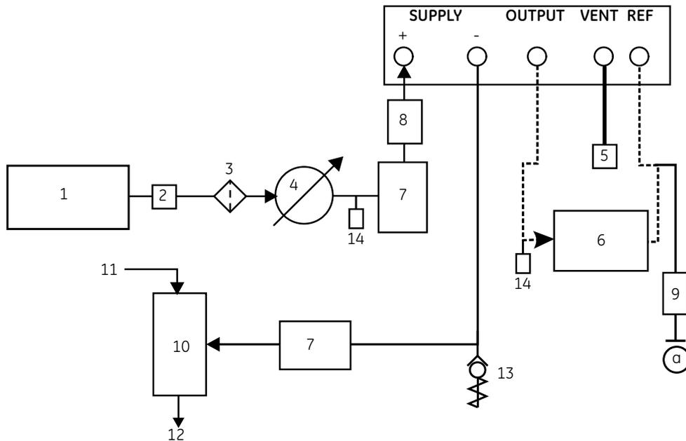
Figure 2-5, Pneumatic Connections with negative gauge pressure generator
