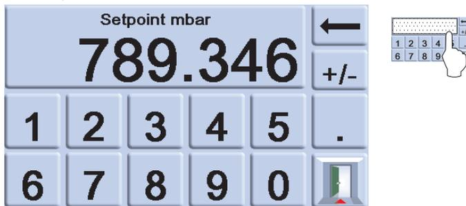
3. If necessary, use the
