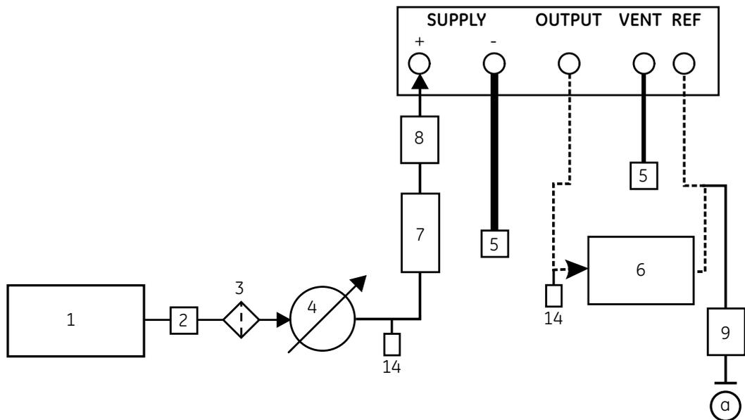
**Figure 2-3, Pneumatic Connections without vacuum supply**
