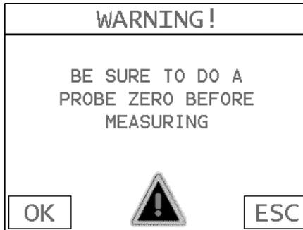
**Note:** When the zero probe option is set to manual, the probe zero disk (battery cap) located on the top of the gauge will be used as a zero standard and the warning screen illustrated above will be displayed.
