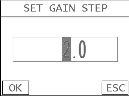
2) Press the
