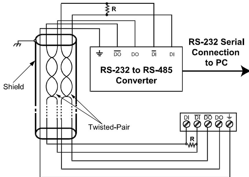
Figure 15. RS-422 or RS-485 Wiring
