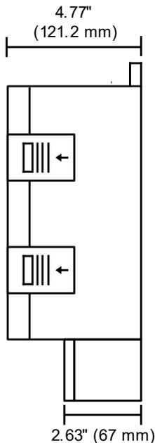
Figure 2. Meter Dimensions - Side View
