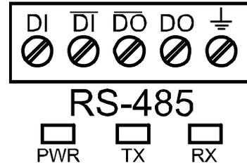
The RS-485 connector has three diagnostic LEDs: a Power (PWR) LED to show when the adapter is powered properly, a Transmit Data (TX) LED to show when the adapter is sending data out from the PC side, and a Receive Data (RX) LED to show when the adapter is receiving data from the meter.
