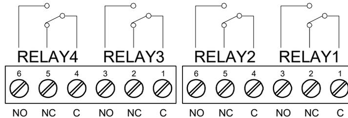
**Figure 12. Relay Connections**
