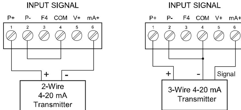
**Figure 9. Transmitters Powered by Internal Supply**
