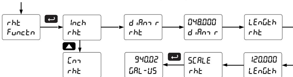
Note: After Scale is displayed continue pressing the Enter button until the meter completes the scaling of the input and display values.
