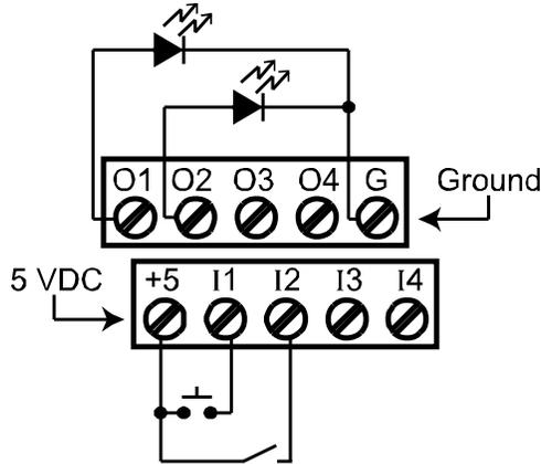
**Figure 19. Digital Input and Output Connections**
