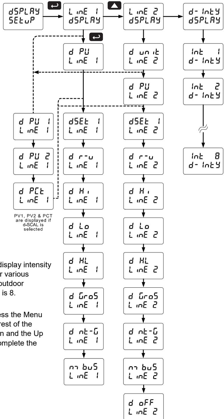
**Display Intensity:** The meter has eight display intensity levels to give the best performance under various lighting conditions. Select intensity 8 for outdoor applications. The default intensity setting is 8.
