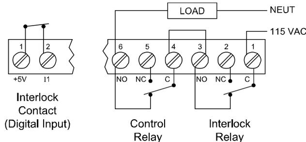
Figure 22. Interlock Connections
