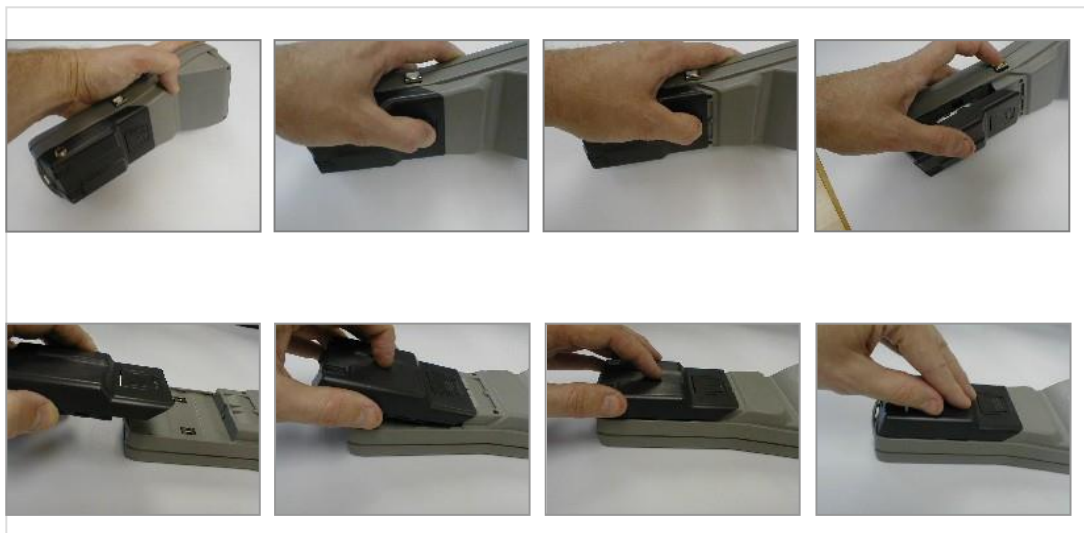
Figure 3.6 – Removing and replacing the battery pack
