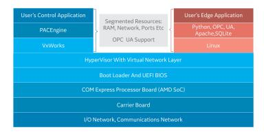
Figure 2. Realtime hypervisor technology provides several cores within a single CPU to enable virtual machines and support both realtime deterministic control and analytic functions simultaneously.
