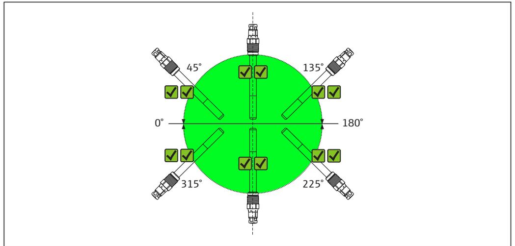
3 Installation angle for Memosens COS81D-\*\*\*\*C\*\*\* (c-shaped spot cap)
