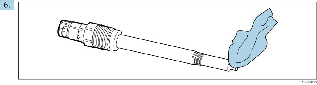
Clean the sensor optics carefully using the cloth provided.
