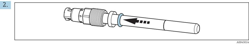
Fit the new O-ring over the spot cap and push it as far as the process connection.
