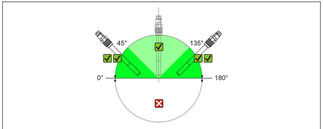
4 Installation angle for Memosens COS81D-\*\*\*\*U\*\*\* (u-shaped spot cap)
