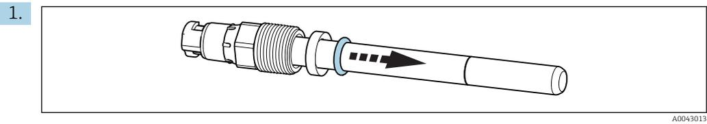
Remove the O-ring on the process connection in the direction of the spot cap.
