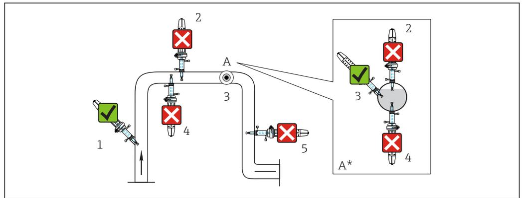
8 Suitable and unsuitable installation positions for Memosens COS81D with u-shaped spot cap and retractable assembly
