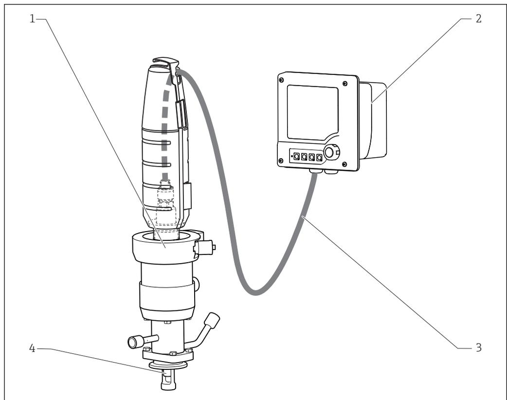
5 Example of a measuring system with COS81D
