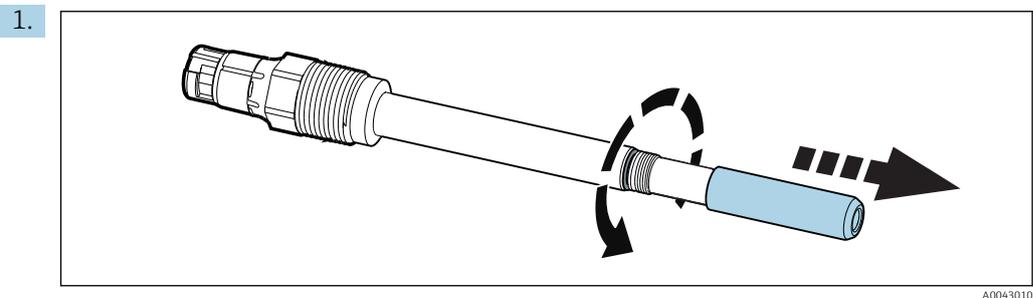
Unscrew the old spot cap and remove.
