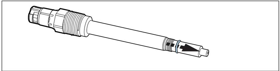
Remove the O-ring above the thread on the shaft.
