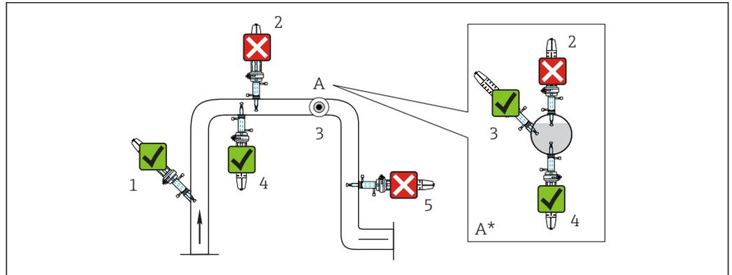
9 Suitable and unsuitable installation positions for Memosens COS81D with c-shaped spot cap and retractable assembly
