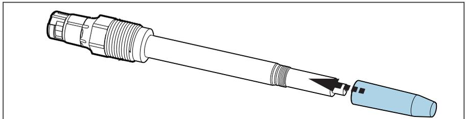
Push the mounting tool from below onto the shaft until it sits over the thread.
