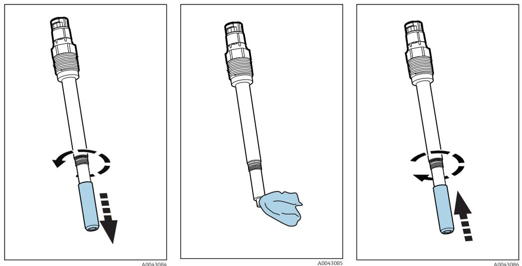
1. Unscrew the spot cap from the sensor head.
