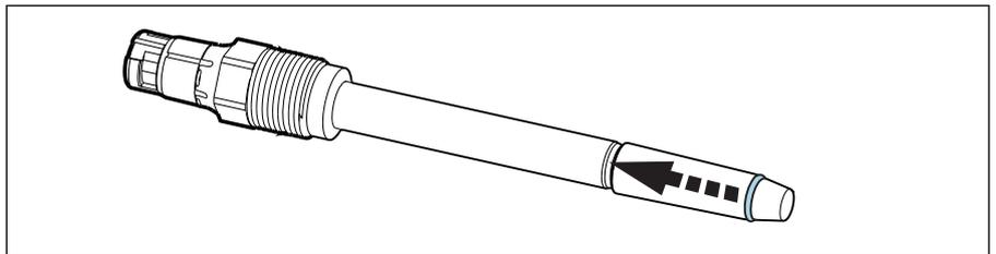
Slide the O-ring over the mounting tool into the position above the thread.
