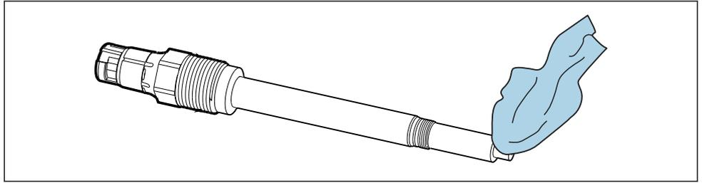
Clean the sensor optics carefully using the cloth provided.
