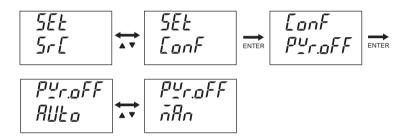
To return to normal mode from setting mode, simultaneously press the CLEAR and ENTER keys. (Press the CLEAR key to go back one level.)
