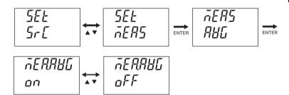
To return to normal mode from setting mode, simultaneously press the CLEAR and ENTER keys. (Press the CLEAR key to go back one level.)
