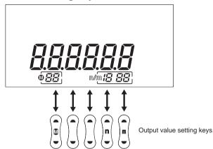
Sets the source output value. Each  $\blacktriangle$  (up) and  $\blacktriangledown$  (down) key corresponds to a digit, and increments or decrements the value by one count. (The  $\blacktriangle$  and  $\blacktriangledown$  marks are used indicate these keys in this manual.) If you attempt to increment or decrement the value 9 or 0, the digit moves up or down one place.
