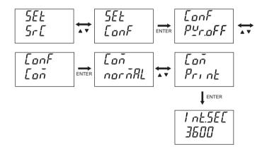
To return to normal mode from setting mode, simultaneously press the CLEAR and ENTER keys. (Press the CLEAR key to go back one level.)
