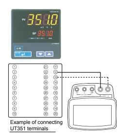
Example of connection: UT351 series temperature controller Connecting method: Connect the source cable of the CA150 to the sensor input terminals of UT (See the following example of connecting measurement input terminals.), and check the indication. Features: The CA150 has many functions, so a single CA150 can be used as an indicator for universal inputs.
