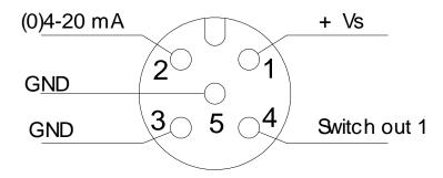
Terminals 3 and 5 are linked internally and can therefore be used either for the output signal or the power supply.
