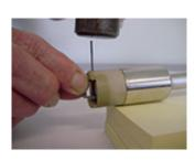
7. Continue to drive the shaft until it is flush with the plastic housing.
