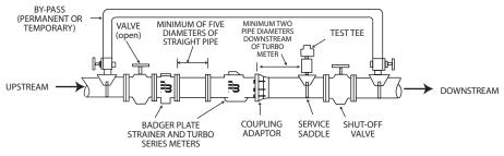
Figure 1: Recommended meter installation
