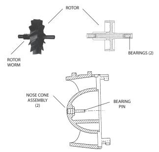
Figure 6: Rotor and nose cone assembly (1-1/2 in., 2 in., 3 in., 4 in. and 6 in. turbo head assemblies)
