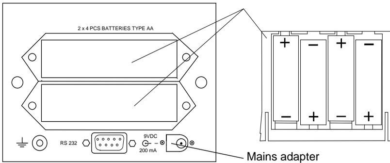
It is also possible to supply the DTI from a mains adapter at the connector shown in the figure above. The mains adapter can be supplied by AMETEK.
