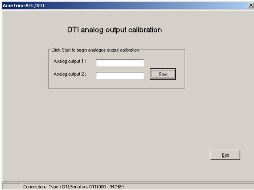
After entering the DTI analog output adjustment window, press “Start” to begin the adjustment procedure.
