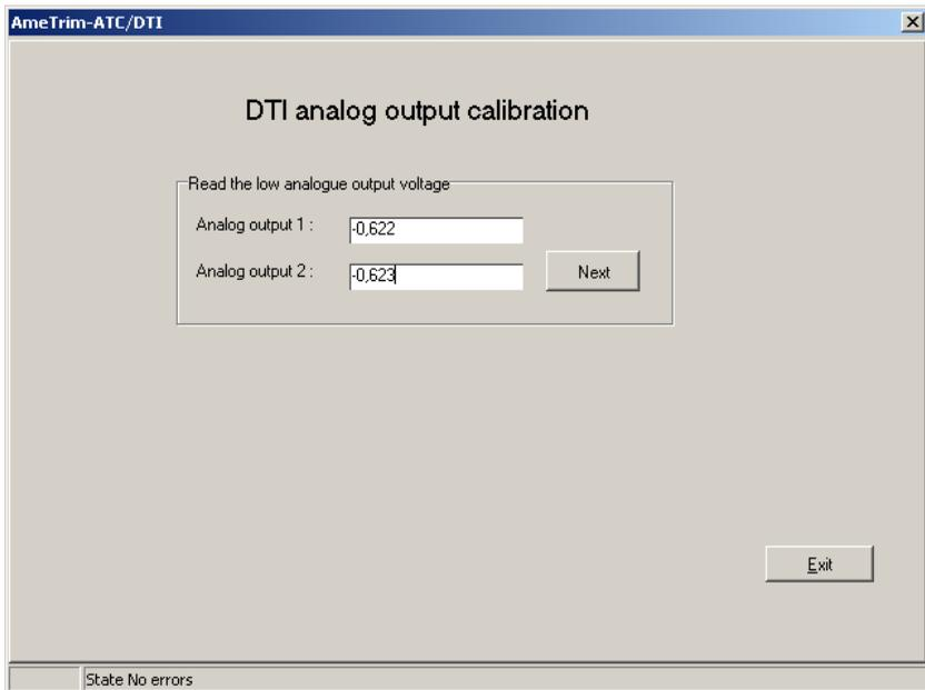
Measure the output voltages of the two analog outputs, enter the values and press “Next”.
