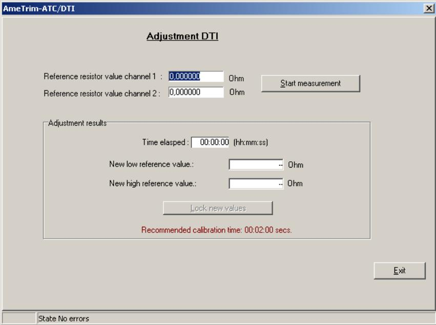
Connect the reference resistors to the input channels and enter the resistor values. Press “Start measurement”, wait until the readings for “New low reference value” and “New high reference value” have stabilized (approx. 2 minutes) and press “Lock new values” to stop the measurement. The locked values can now be downloaded to the DTI or cancelled.
