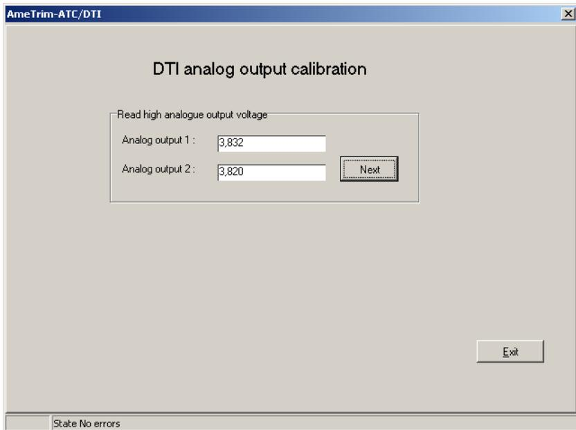
Repeat the measurement of the output voltage for high output, enter the values and press “Next”.
