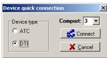
Select “DTI” and “Comport” in the “Device Quick Connect” dialog box and press “Connect”. If the DTI is not switched on or is not connected to the selected port, then the software returns to the Ametrim adjustment software main menu.
