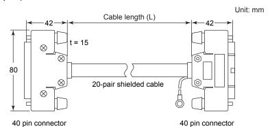
KS1: L = 1 m, 2 m, 3 m, 5 m, 7 m or 10 m, up to 50 m in 5 m increments
