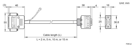
Note: An FG connection wire is attached to the other side connector of the AKB131 and AKB132 cables.
