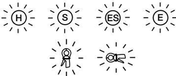
This flashing indicates that a terminal or a current clamp needs to be either connected or disconnected. You must correct the connections or the measurement will not proceed. The flashing of terminal H may also indicate that current  $I_{H,E}$  is too low. The flashing of terminal S may also indicate that resistance  $R_s$  is too high. The flashing of terminal ES may also indicate that the current  $I_{ES}$  measured by the clamp is too low.
