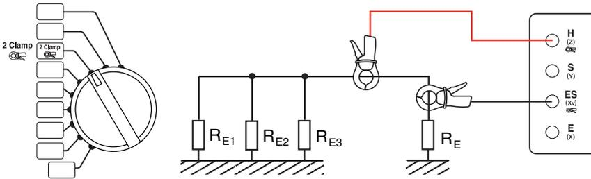
Observe the following minimum distances between the two clamps in order to avoid direct electromagnetic influences between the transmitting clamp and the receiving clamp:
