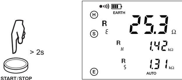
**NOTE:** Repeat the process at 52% and at 72% for the S electrode.
