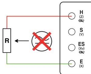
3. The 6472 makes a measurement with a positive current (R+), then reverses the direction of the current and makes another measurement with negative (R-).
