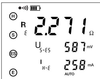
4. To display the measurement parameters, press **DISPLAY** several times.
