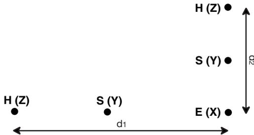
If you find the same values, your measurement is reliable. If the measured values are substantially different, it is likely that they were influenced by earth currents or a groundwater source. It may be useful to drive the electrodes deeper and/or wet the ground near them to reduce their contact resistance with the soil.
