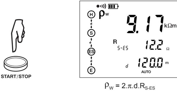
To display the measurement parameters, press **DISPLAY** several times.
