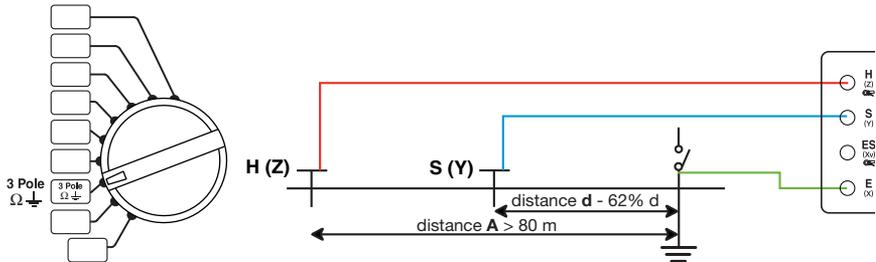
In order to avoid electromagnetic interference, it is best to unwind the full length of each cable from the reel, to keep the cables as far apart as possible on the ground, taking care not to form loops, and to avoid placing the cables near or parallel to metallic conductors (cables, rails, fences, etc.).
