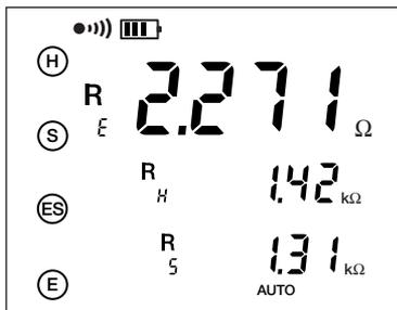
We recommend repeating the measurement with the auxiliary electrodes placed at a different distance and in another direction (see § 5.4.3).
