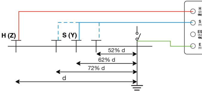
The 3 measurement results should be the same to within a few percent. If this is the case, the measurement is valid.
