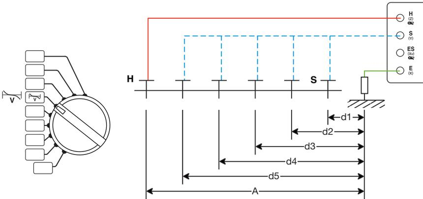
In order to avoid electromagnetic interference, it is best to unwind the full length of each cable from the reel, to keep the cables as far apart as possible on the ground, taking care not to form loops, and to avoid placing the cables near or parallel to metallic conductors (cables, rails, fences, etc.). Connect the cables to terminals **H (Z)** and **S (Y)** and connect terminal **E (Z)** to the earth.
