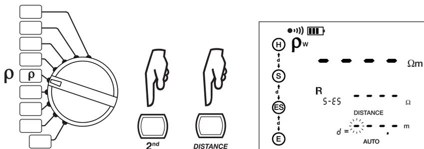
3. To modify the hundredths (of meters or feet), press the ▲ button until the desired digit is displayed (0-9).
