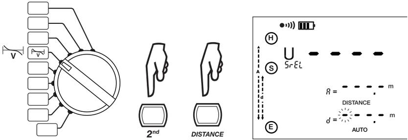
4. To modify the hundredths (of meters or feet), press the **▲** button until the desired digit is displayed (0-9).
