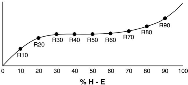
Take the average of the 3 or 4 readings on the plateau to obtain the earth electrode resistance.
