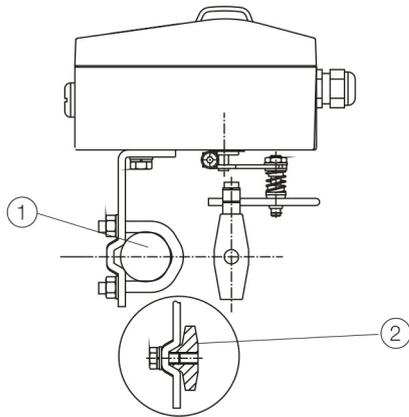
① Columnar yoke                      ② Cast iron yoke
