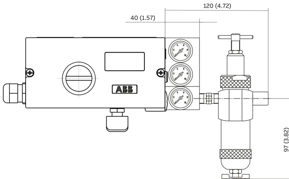
Figure 19: Positioner TZIDC with mounted pressure gauge block and filter regulator
