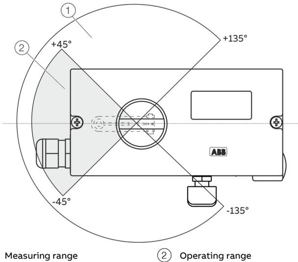
Figure 11: Measuring and operating ranges of the positioner
